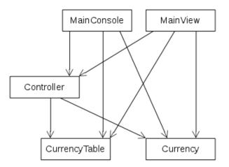
That is the model layer's classes do not know neither the controller layer or view layer and the controller layer knows nothing about the view layer. The result is that you can replace the view layer without it affects the rest of the program.
