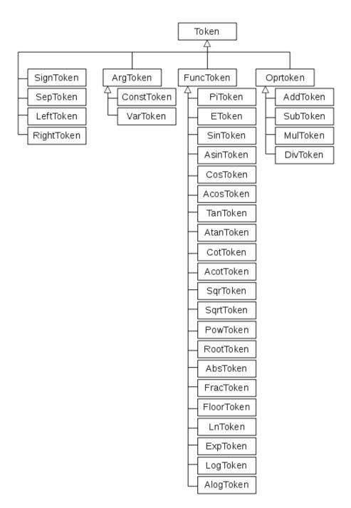
It is very simple classes, and as an example is *SinToken* a class that represents a sine function. The class is derived from *FuncToken*, and the class has only two properties, where the first returns the number of arguments, while the second determines the function's value from a single argument:
