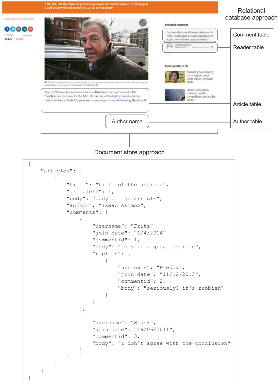
Figure 6.13 Document stores save documents as a whole, whereas an RDMS cuts up the article and saves it in several tables. The example was taken from the Guardian website.
