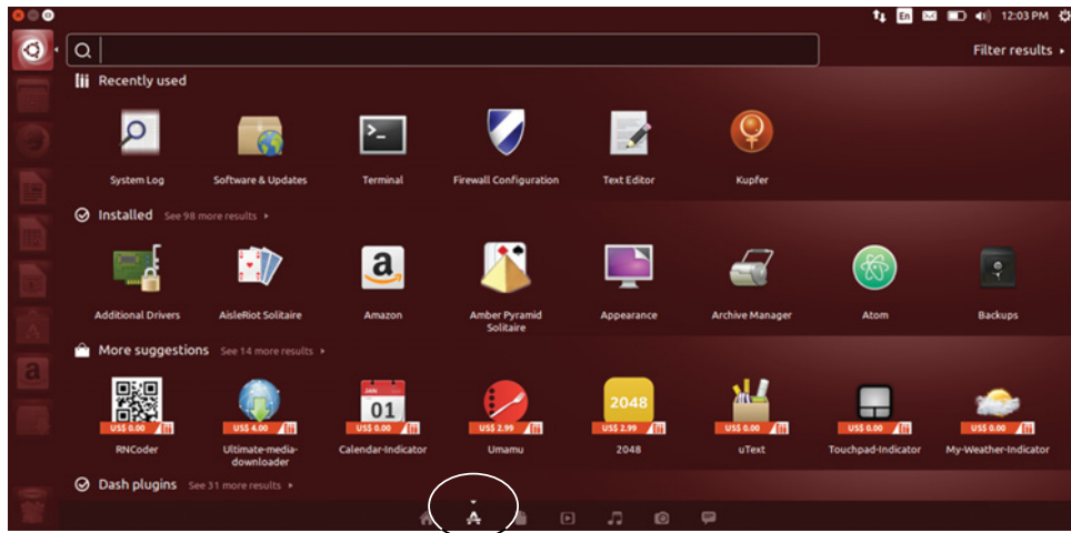
Figure 6.3 You can ask Unity to search only through programs on your computer using the Application scope on the Dash screen.
