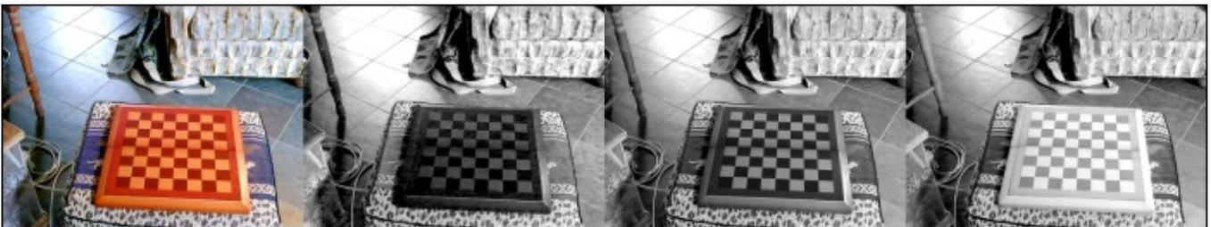
Note that the red channel captures the checkerboard brightly and with good contrast between lighter and darker squares. Moreover, the board's border appears quite light. This is good because we are soon going to use a detector that is optimized for a black-and-white board with a white border.
