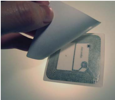
FIGURE 11-1: The internal components of an RFID sticker
