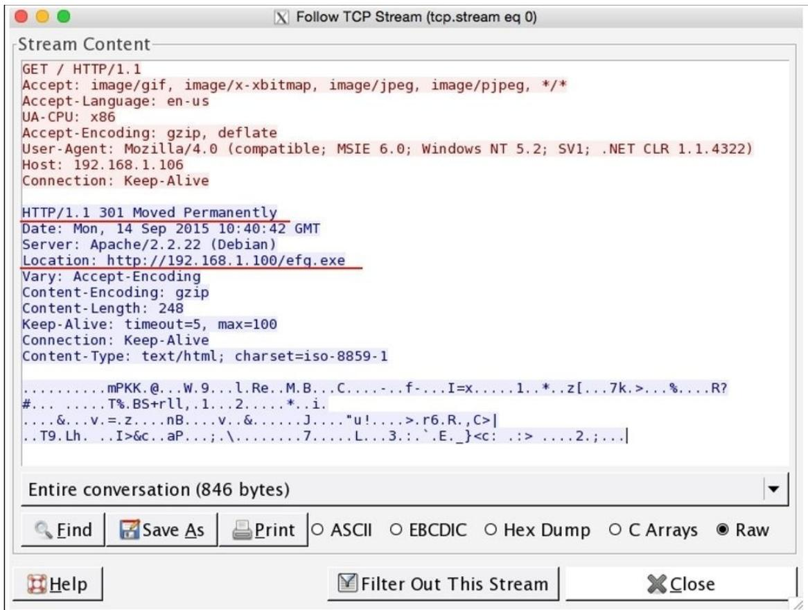
Figure 7.21: TCP stream between the client and real (compromised) server
