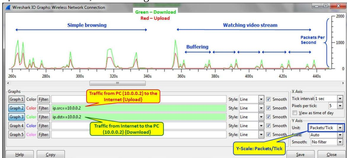
In the first graph, we see that we've measured the traffic when the X Axis is configured to a tick interval of one second and the Y-Axis scale is configured to packets/tick. The result that we've got is that while browsing (on the left-hand side of the graph) or while watching a movie (on the right-hand side of the graph), the upload and download traffic is nearly identical.
