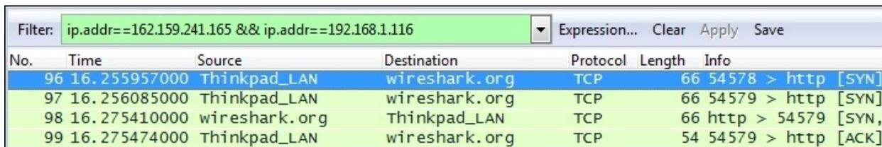
This particular display filter syntax works with IP addresses, not with hostnames, and uses an `ip.addr==` (IP address equals) syntax for each node along with the `&&` (and) logic operator to build a string that says display any packet that contains this IP address *and* that IP address. This is the type of display filter that you will be using a great deal for packet analysis.
