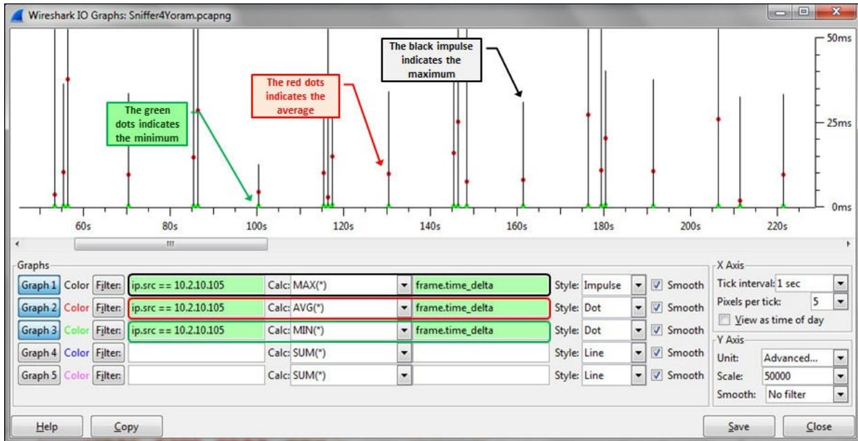
What we see in the screenshot is a graph of the minimum, average, and maximum time delta between frames. What do we do with it and how do we use it for network debugging? This will be covered in [Chapter 10, HTTP and DNS](#).
