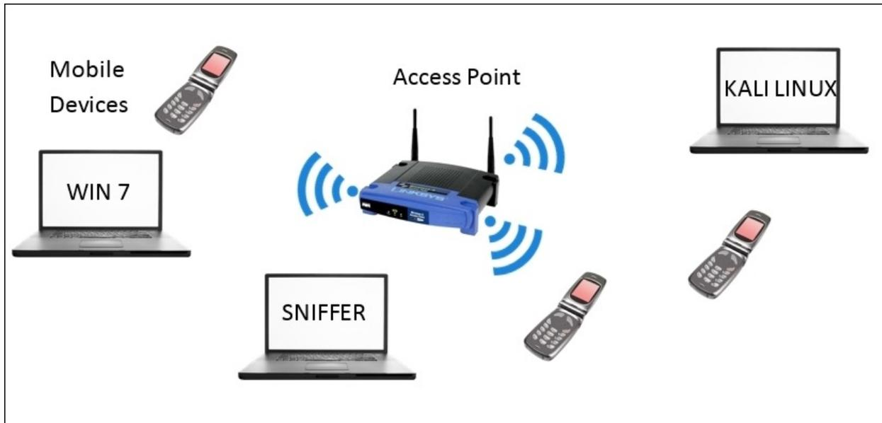
Hopefully, now you have a rough idea about my internal network that I'll be working with. The access point located at `192.168.1.1` assigns the IP address to all these devices using DHCP (the DHCP range starts from `192.168.1.100` and continues up to `192.168.1.110`; it means I can have a maximum of 10 DHCP clients at one instance). For this chapter, the IP address for our attacking machine is static assigned to `192.168.1.106`.
