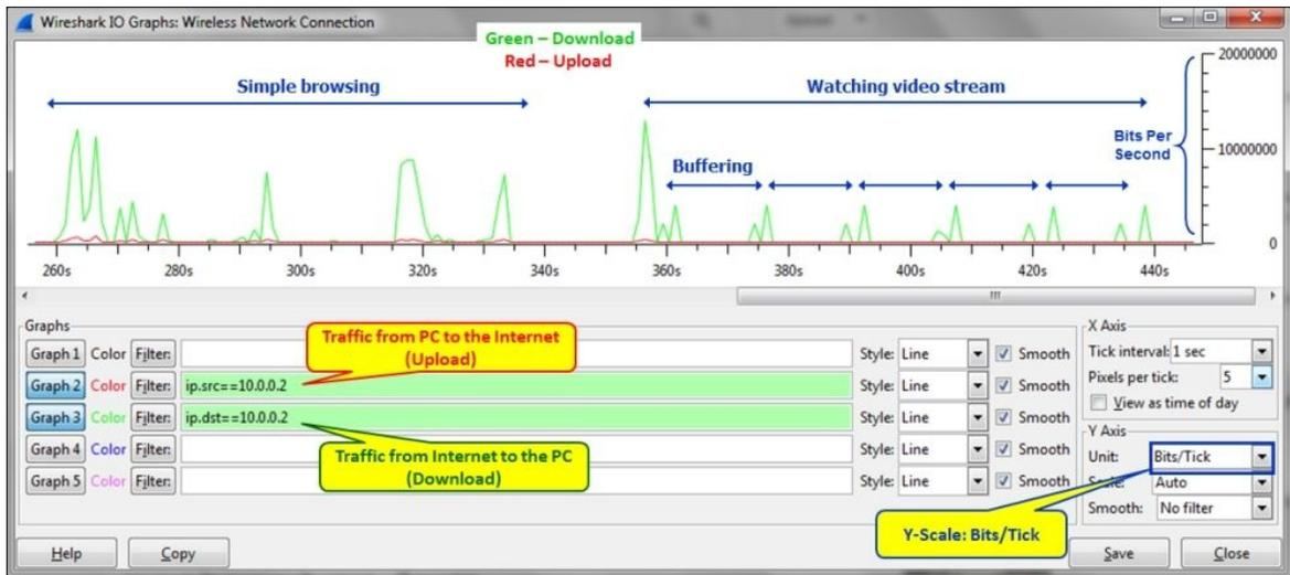
In the second graph, we see the traffic in bits/sec. Here, we see the bandwidth required from the network while using it to connect to the Internet; that is, an asymmetrical bandwidth when most of the traffic is in the download direction.
