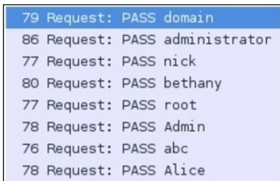
A screenshot of a network traffic capture tool showing FTP traffic. The traffic is filtered to show only 'PASS' requests. The list of requests is as follows:
