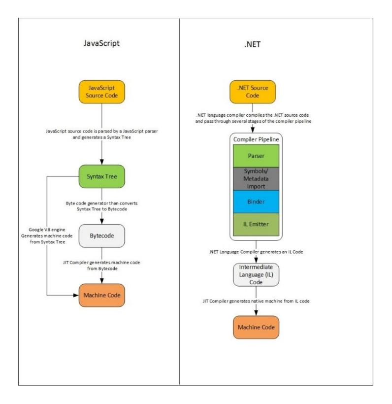
The JavaScript parser parses and tokenizes the JavaScript code into a syntax tree. All the browsers, except Google V8, parse the syntax tree and generate a bytecode that finally converts into a machine code through JIT compilation. On the other hand, Google V8 engine parses the syntax tree and instead of generating a bytecode first, it directly generates the machine code.
