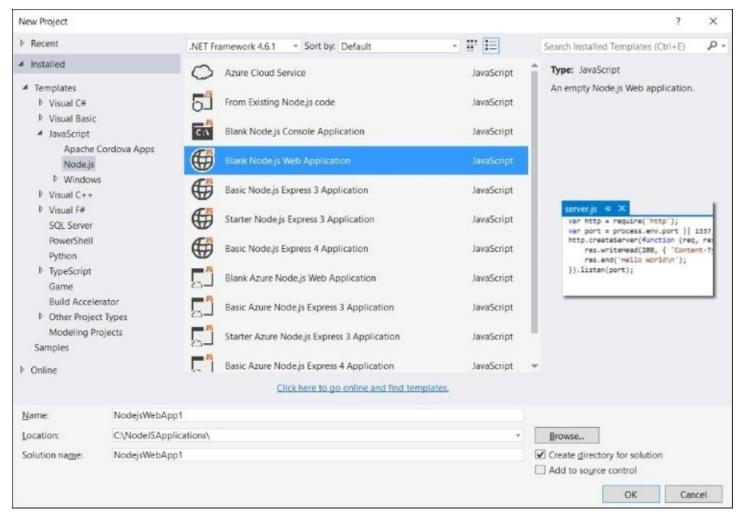
A blank Node.js application template creates one server.js file and sets the main attribute in the package.json file to load server.js. The content of server.js is as follows:
