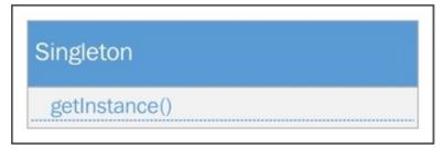
In a singleton pattern, the constructor should be private which restricts the user to create objects using a new keyword and exposes one method that creates an instance and verifies that only one instance exists. A simple example could be a logger object that writes the log to the browser's console window:
