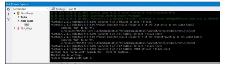
In our product.test.js test script, we have two tasks. One is to check whether passing the string values to one of the two elements such as txtProdUnitPrice and txtProdQuantity will return 0. As our product.js file does not handle this condition, it will give an error.
