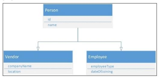
In order to articulate the same inheritance using the JavaScript constructor function approach, we can use the prototype property of both Vendor and Employee to the person object, as shown in this code:
