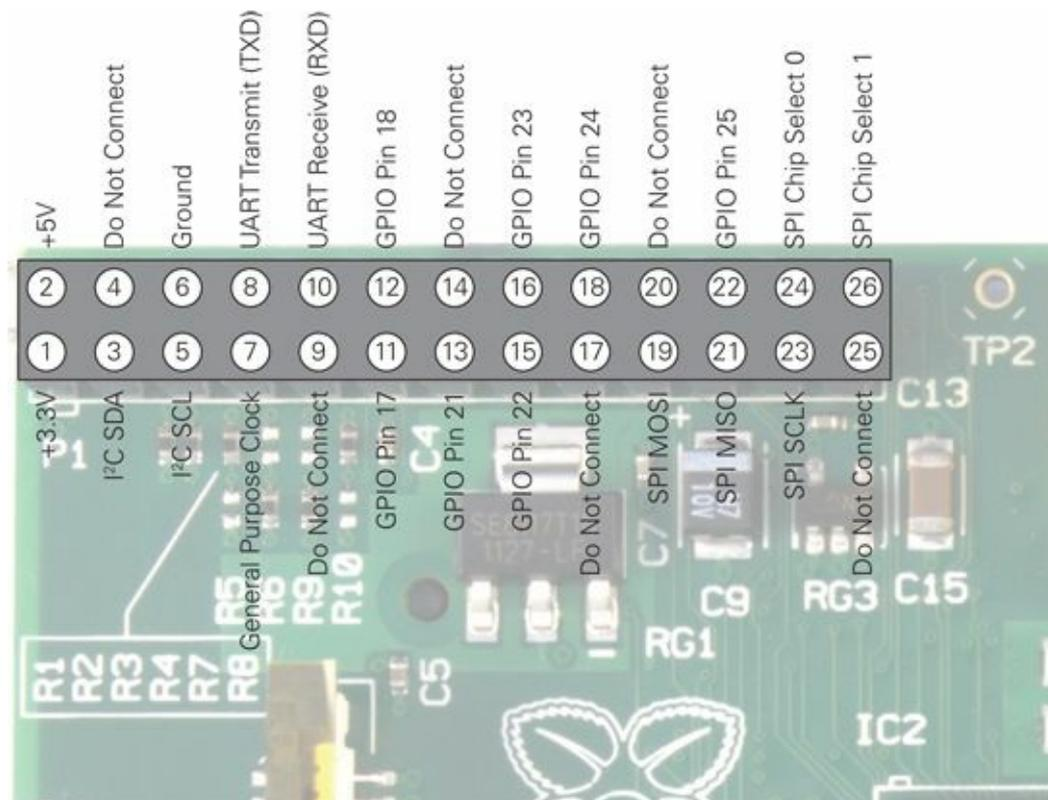
Pin numbers for the GPIO port are split into two rows, with the bottom row taking the odd numbers and the top row the even numbers. It’s important to keep this in mind when working with the Pi’s GPIO port: most other devices use a different system for
