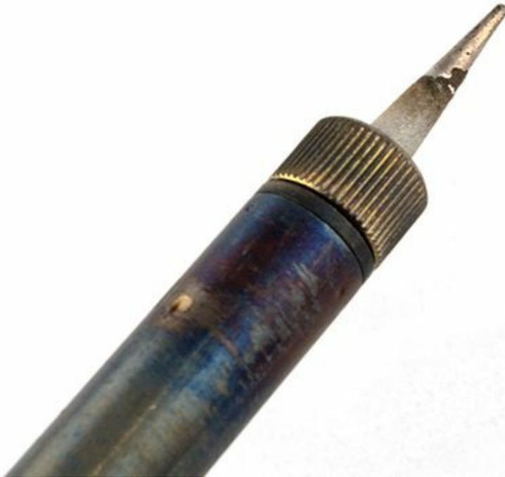
This process of tinning the tip protects it against damage and ensures that it will efficiently transfer heat onto the surfaces to be soldered. Failure to properly tin the iron's tip is one of the most common causes of bad solder joints. You may need to repeat this process more than once if you're soldering a lot of connections, and you'll need to do it again at the end of the soldering session. In general, if the tip of the soldering iron loses its shiny coating, repeat the tinning process.
