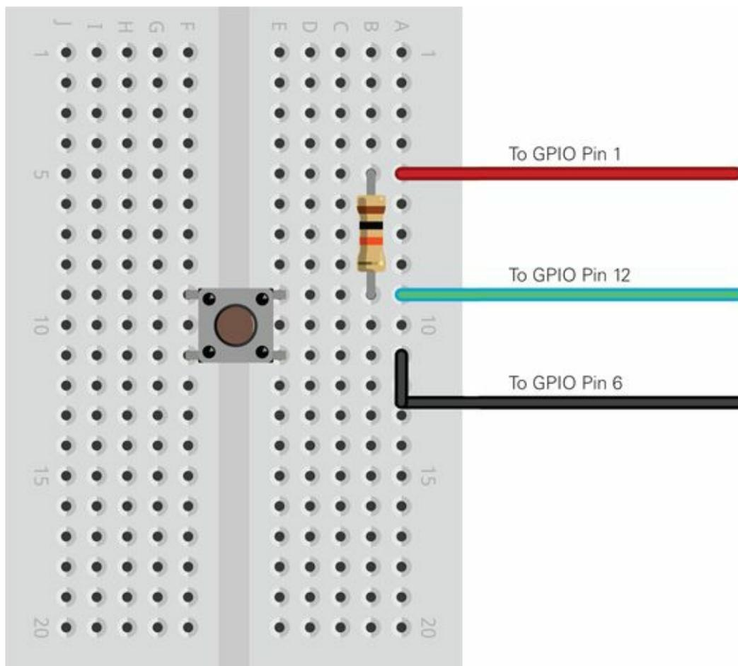
The circuit you just built creates a situation whereby the input pin, which in this instance is Pin 12 of the Raspberry Pi's GPIO port, is constantly high thanks to the pull-up resistor connected to a 3.3 V supply. When the push-button is pressed, the circuit is grounded and becomes low, providing the cue for your Python program to know that the button has been activated.
