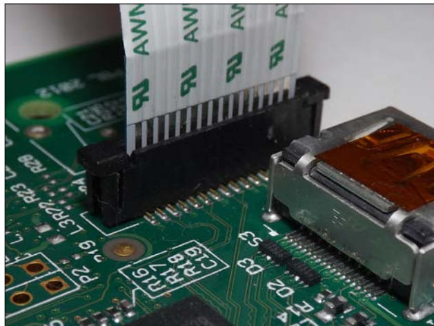
The ribbon connector for the camera module is located next to the HDMI socket
