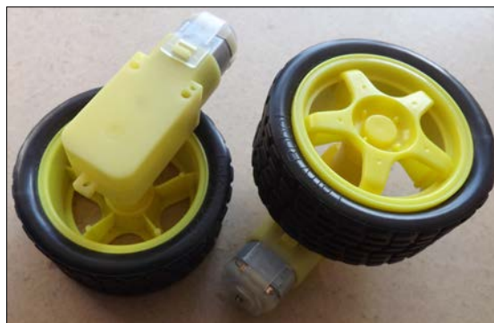
These wheels with built-in geared motors are ideal for small rovers
