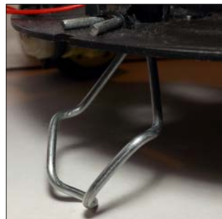
Wire skid fitted to the front of the Rover-Pi robot
