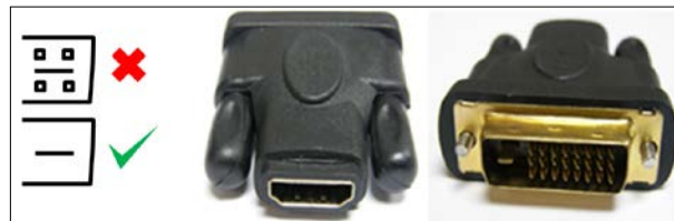
HDMI to DVI connection (DVI-D adaptor)
