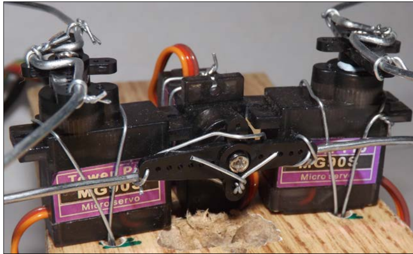
The servos are mounted upside down on the underside of the board
