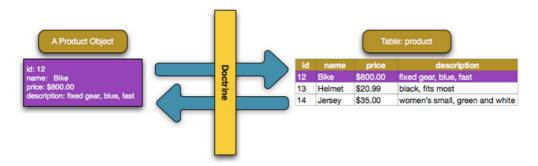
For Doctrine to be able to do this, you just have to create "metadata", or configuration that tells Doctrine exactly how the Product class and its properties should be *mapped* to the database. This metadata can be specified in a number of different formats including YAML, XML or directly inside the Product class via annotations:
