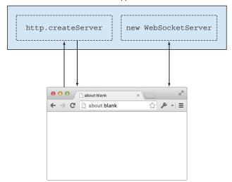
Figure 9.6 A Node web application should support both standard HTTP requests and WebSockets.
