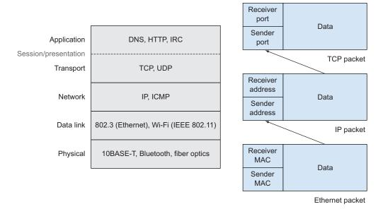
Figure 7.1 Protocols are grouped into seven logical layers. Packets are wrapped by protocols at consecutive layers.
