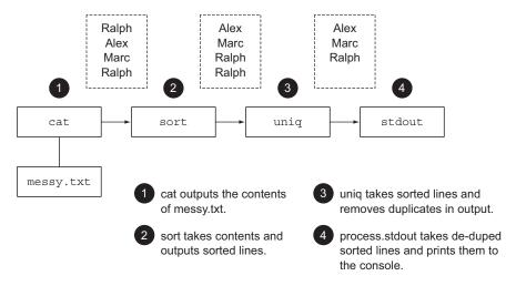
Figure 8.5 Stringing external applications together with spawn
