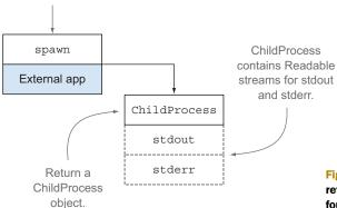
Figure 8.4 The spawn method returns a streaming interface for I/O.
