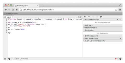
Figure 11.3 Node inspector connected to the debugger
