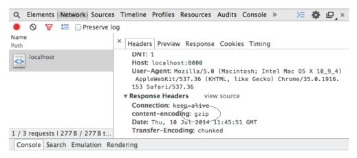
Figure 5.3 The network inspector confirms the content was compressed.
