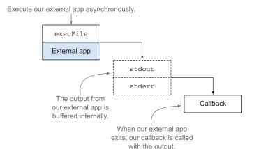
Figure 8.2 The execFile method buffers the result and provides a callback interface.
