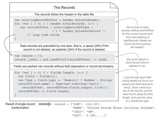
Figure 3.8 The records: transformation from the specification to code using the Node Buffer API
