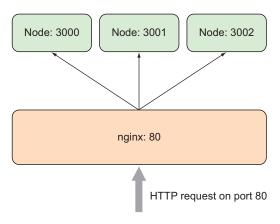
Figure 12.6 A Node program running alongside Apache or nginx
