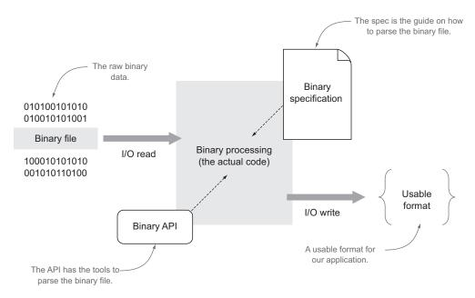
Figure 3.3 The transformation of binary data into a more usable/programmable format
