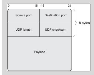
The UDP header is 8 bytes, followed by an optional payload of up to 65,507 bytes for IPv4 and 65,527 bytes for IPv6.
