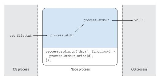
Figure 2.2 Data flows in a simple program that uses stdio.
