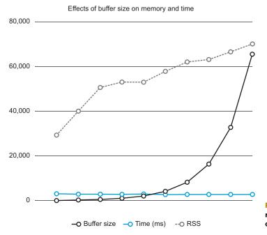
Figure 5.5 A graphical representation of the memory usage of streams
