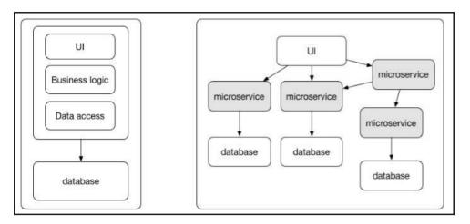
As you can see on the previous diagram, the monolithic application differs totally from an application created using the microservices architecture. Let's compare the two approaches and point out their advantages and flaws.
