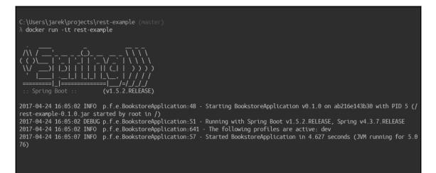
That wasn't very tricky, right? The basic Dockerfile contains just three lines, the base image definition using FROM, COPY to transfer the executable jar into the image's filesystem, and a CMD instruction to run the service.
