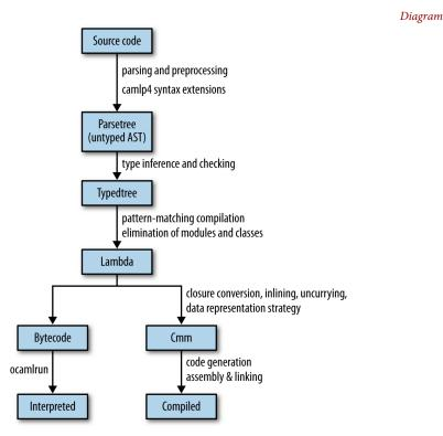
Notice that the pipeline branches toward the end. OCaml has multiple compiler backends that reuse the early stages of compilation but produce very different final outputs. The *bytecode* can be run by a portable interpreter and can even be transformed into JavaScript (via js\_of\_ocaml) or C source code (via OCamlCC). The *native code* compiler generates specialized executable binaries suitable for high-performance applications.
