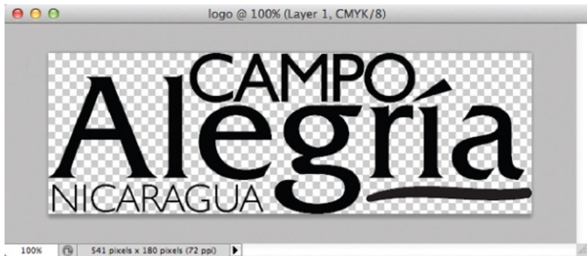
Figure 8-2 When a file with transparency is displayed in a graphics program, you typically see a gray and white checkerboard in the transparent areas of the image.
