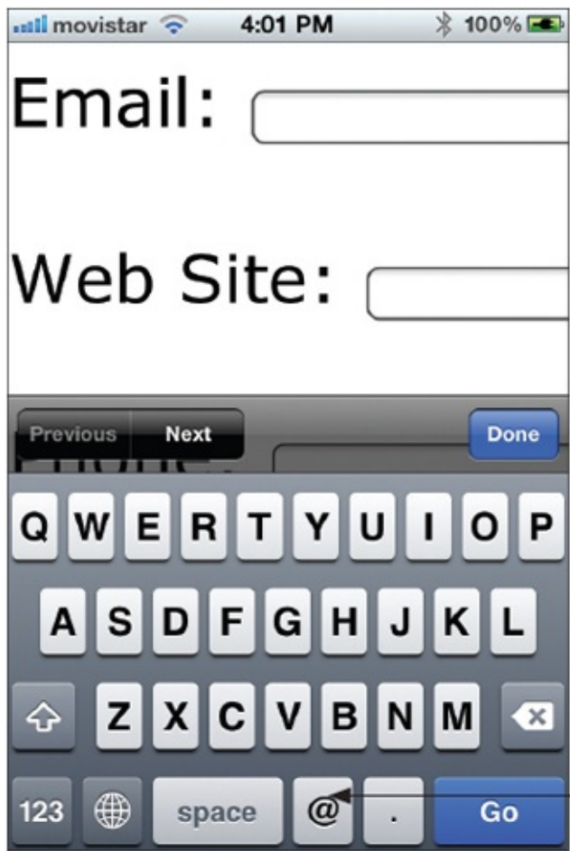
Figure 12-5 Keyboard adjusted to help user input email addresses
