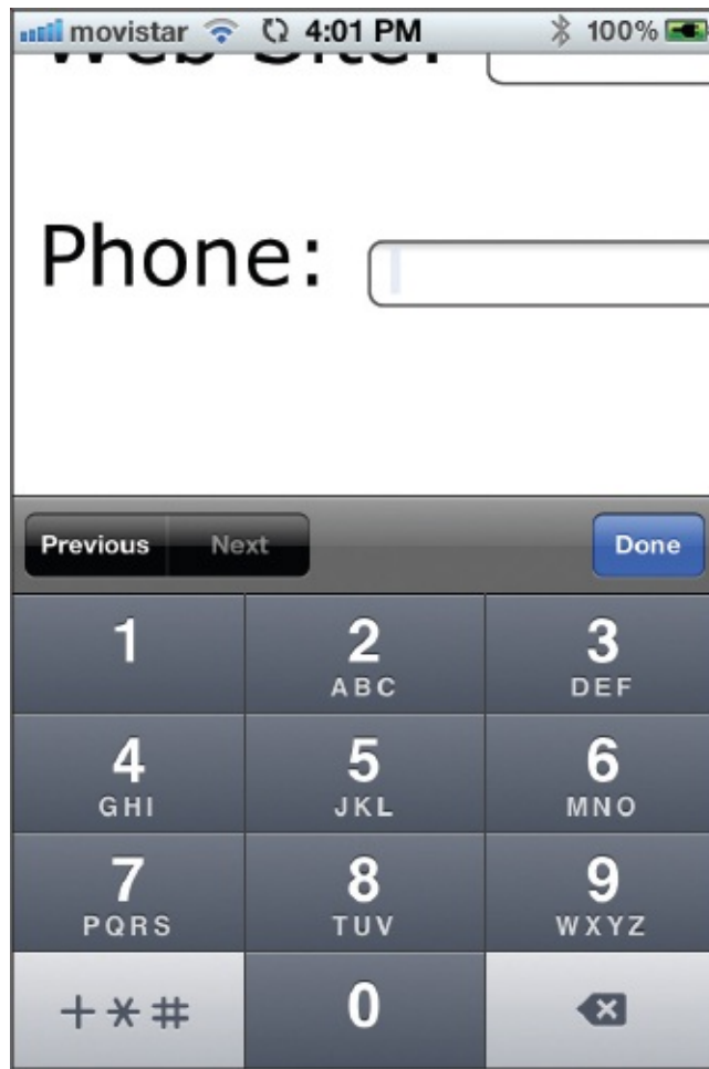
Figure 12-7 Keyboard adjusted to help user input phone numbers
