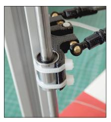
FIGURE 12-18: A carriage fitted to a rod on a 3DR printer.
