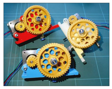
FIGURE 14-5: The 3D-printed geared extruder has more parts to assemble but can produce greater power and faster printing.
