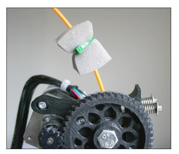
FIGURE 14-22: A piece of dry sponge keeps fluff, grease, and dust from entering (and jamming) the tiny nozzle of your hot-end.
