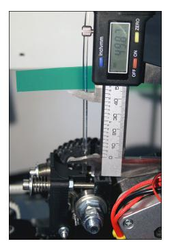
FIGURE 15-21: Use a digital micrometer to measure the distance that the input filament moves when 20mm is extruded.
