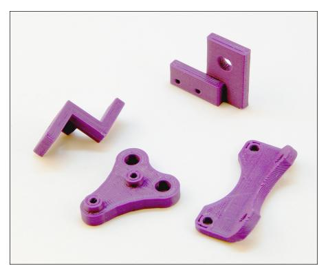
FIGURE 5-1: Four brackets for electronics that are printed to complete the MendelMax 2.0 RepRap 3D-printer kit.
