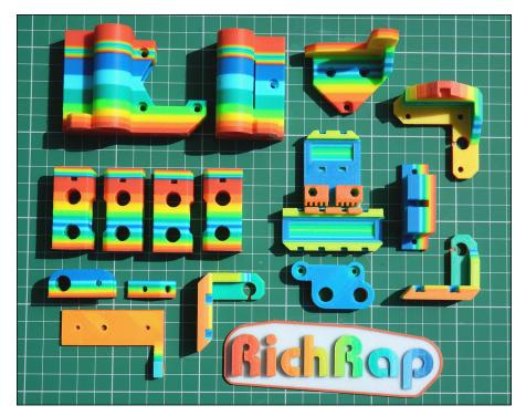
FIGURE 14-20: Continuous multicolor printing via the cut-and-follow-on method.
