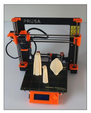
FIGURE 10-21: The Prusa i3 MK2 3D printer is one of the world's most imitated RepRap 3D printers.
