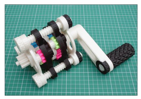
FIGURE 15-8: A multistage planetary gearbox. Home 3D printers can make all the parts, but some assembly is still required.
