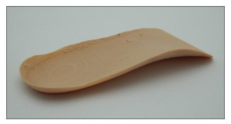
FIGURE 10-15: 3D-printed soft insole.
