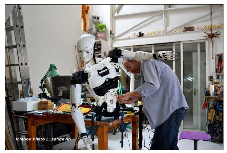
FIGURE 17-3: The InMoov 3 printed humanoid project in construction.
