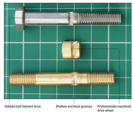
FIGURE 14-1: Typical filament drives used in thermoplastic extruders.
