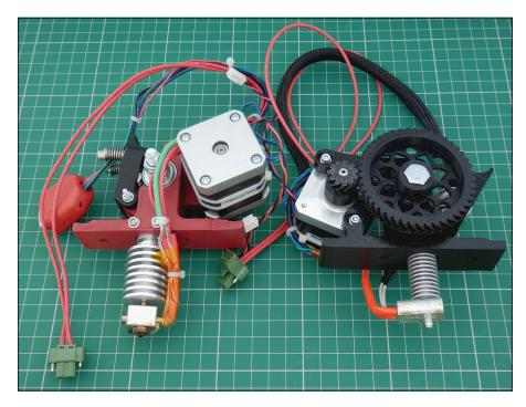
FIGURE 14-9: RepRap extruder designs.
