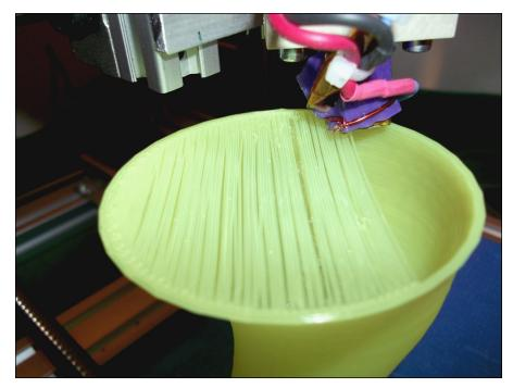
FIGURE 14-24: Bridging a filament. With good cooling and a few alternating layers, the spanned first layer becomes a solid surface that can be printed on after a second bridging layer in the opposite direction.
