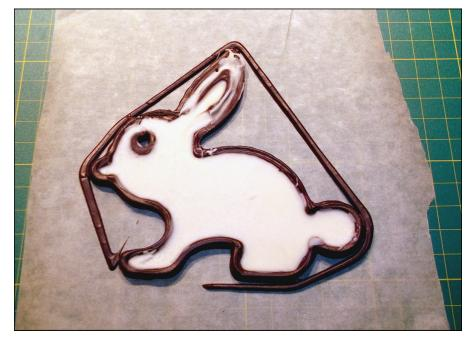
FIGURE 4-5: 3D-printed white-and-dark chocolate bunny, created with a RepRap 3D printer and Richard's Universal Paste Extruder. Other alternatives use fused filament fabrication (FFF, which is another term for the proprietary term FDM, which is owned by Stratasys Corp.) with wax and granular materials in paste form such as sugar, salt, and some ceramic powders that are compatible with sintering and granular binding fabrication.
