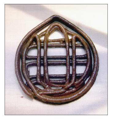
FIGURE 14-13: Printing chocolate muffin mix requires a basic syringe without a needle, which provides a 3mm bead of extrusion. Pastas and fondants make for great food-based 3D-printing experiments. Masa flour (used to make corn chips) is a perfect food for 3D printing: It sticks to itself, and after it's extruded onto a baking tray or silicon sheet, you can bake it for the ultimate custom-designed crunchy treat (see Figure 14-14).
