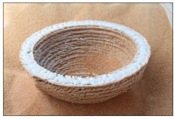
FIGURE 7-1: A bowl from the SolarSinter created from sand and sunlight.
