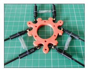
FIGURE 12-19: The 3D-printed main platform of a 3DR delta printer.
