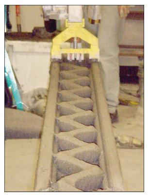
FIGURE 3-7: Corrugated wall made of 3D extruded concrete.
