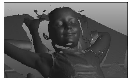
FIGURE 5-10: Software stitching together multiple scans of the reclining subject. Hair doesn't scan well and requires sculpting before printing.
