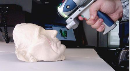
FIGURE 6-3: A FARO laser arm creating a 3D model of this life mask.
