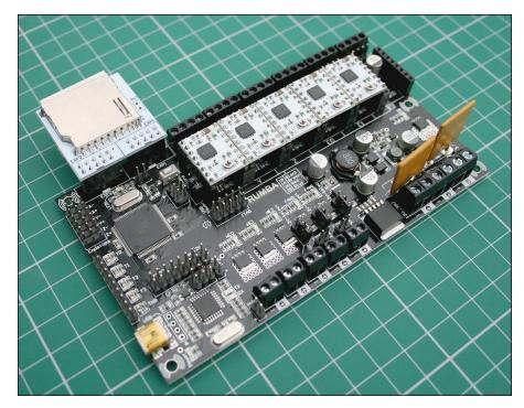
FIGURE 13-5: RUMBA with an expansion adapter for a memory card to store model G-code, ready for printing.
