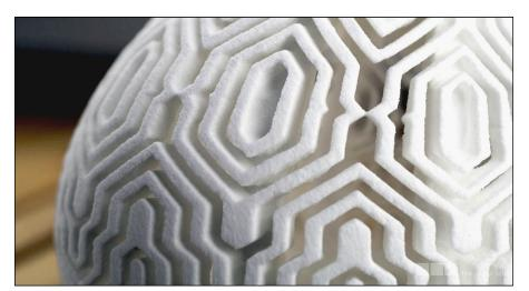
FIGURE 4-7: 3D printing with bound sugar granules.
