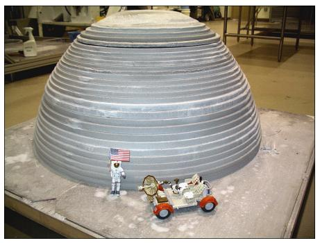
FIGURE 3-14: A small-scale lunar habitation printed from concrete.
