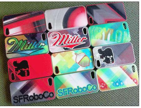
FIGURE 14-19: These iPhone cases are fine examples of layer-selective color printing that uses a single extruder.
