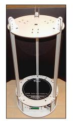
FIGURE 12-12: During assembly, aluminum extruded sections are fitted to achieve vertical height for the delta printer.
