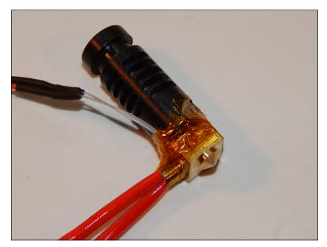
FIGURE 10-8: A standard J-head-style FFF/ FDM extruder hot-end.
