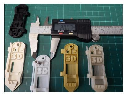
FIGURE 16-3: Printing a number of calibration models helps you refine settings for different materials and nozzle sizes.
