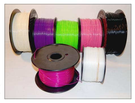
FIGURE 4-1: Spools of thermoplastic filament of various materials.
