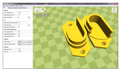
FIGURE 16-8: The key settings are shown here in Cura.
