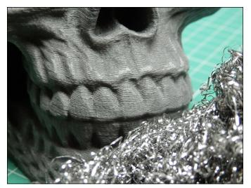
FIGURE 16-10: A 3D-print object being polished.
