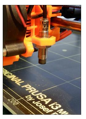
FIGURE 12-22: A noncontact P.I.N.D.A. probe sensor fitted to an assembled Prusa i3MK2 3D printer.
