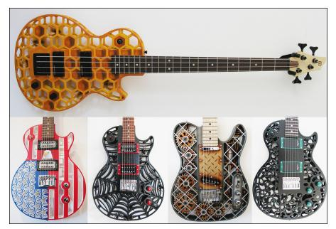
FIGURE 9-2: Olaf Diegel's custom 3D-printed guitar bodies for fully functional electric instruments.
