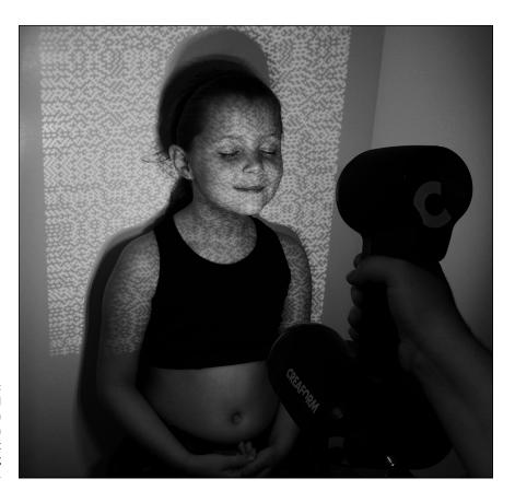
FIGURE 5-9: A handheld Creaform Go!Scan structured-light scanner capturing a human face.
