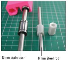
FIGURE 12-5: The rods and bearings used in a 3D printer allow the carriage or axis to slide smoothly along or up and down.
