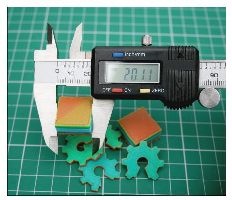
FIGURE 15-24: Make sure that your printed cube measures correctly.
