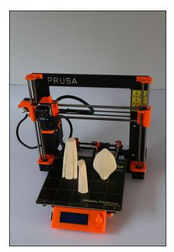
FIGURE 16-14: Sections of the tail scaled up 600 percent and cut into sections, then printed as a plate of parts to be glued back together after 3D printing.
