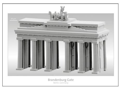
FIGURE 2-4: Object created via multiphoton lithography on a NanoScribe 3D printer.
