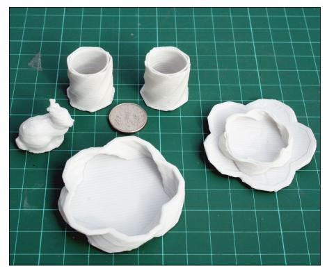
FIGURE 11-15: Fine porcelain clay can be printed with a paste extruder and then fired in a normal kiln to produce ceramic.
