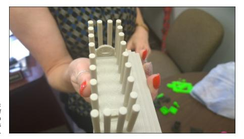
FIGURE 8-1: Example of 3D-printed design for centrifuges used in schools.
