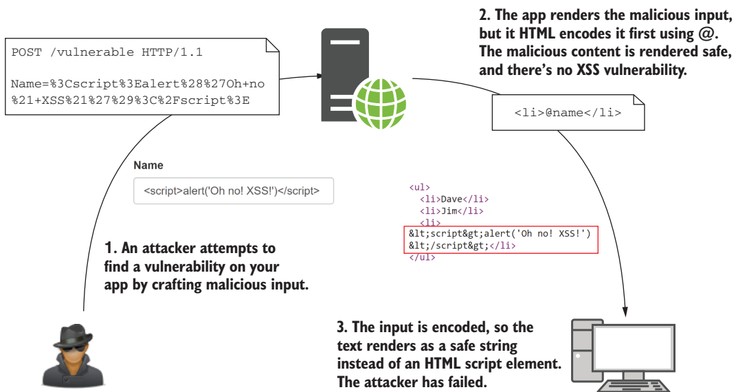
Figure 18.8 Protecting against XSS attacks by HTML encoding user input using @ in Razor templates
