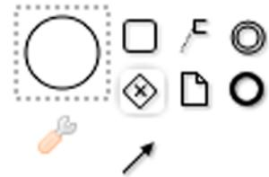
**Figure 3.3** A context menu from the modeling pane in the Activiti Modeler, which enables you to quickly draw tasks, gateways, events, and sequence flows
