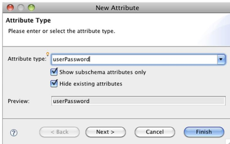
**Figure 10.6** Adding a new userPassword attribute to complete the credentials for the newly created user entry
