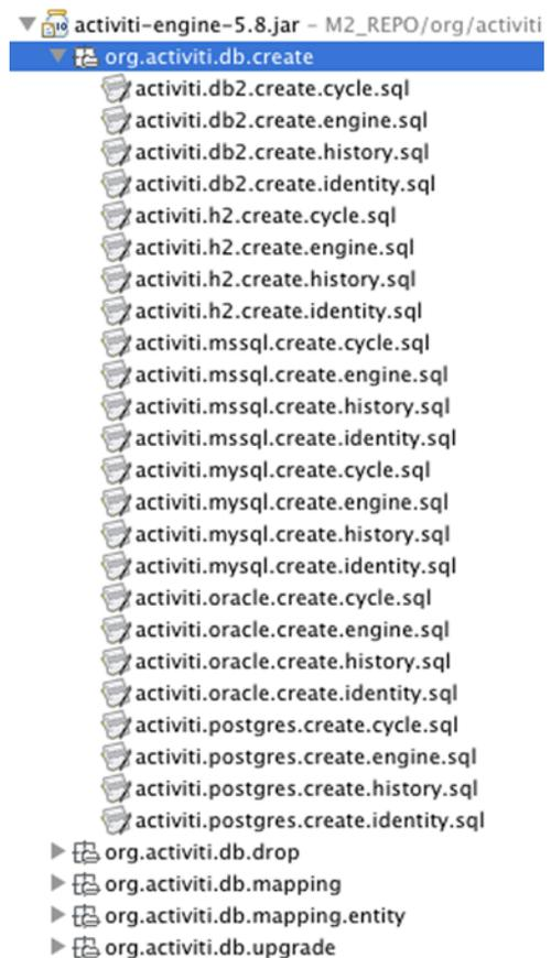
**Figure 15.4** The database scripts in the Activiti Engine JAR in Eclipse
