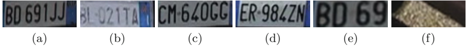
Fig. 7. Extraction step on ACS Video Dataset: examples of correct ((a)–(d)), partial (e), and wrong (f) extracted ROIs
