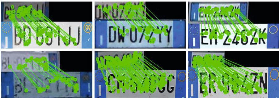
Fig. 8. Recognition step: license plates extracted by the ACS Video Dataset (top of each figure) and correctly matched with license plates of the ACS Recognition Dataset (bottom of each figure). Green circles indicate keypoints common to the matched images and green lines connect matched keypoints.
