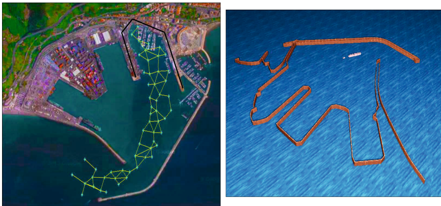
Fig. 1. Left: Satellite photo of the port of Salerno. We focus our attention to the right dock (indicated with black lines) where small vessels as motorboats and sailboats are allowed to land or depart (the other two major docks on the left are only for container or cargo ships). On the same image the ITM on which the events are gathered is superimposed. The green lines connect the neighbor nodes, and for each node we define the correspondent zone as the locus of points that are closer to that node, with respect to the others. Right: A picture taken from the simulator used in this paper, that accurately reproduces the shape of the port and generates realistic trajectories of ships in the area.
