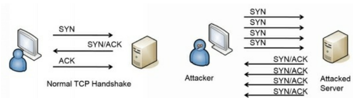
Figure 7.2: TCP handshake and SYN flood attack
