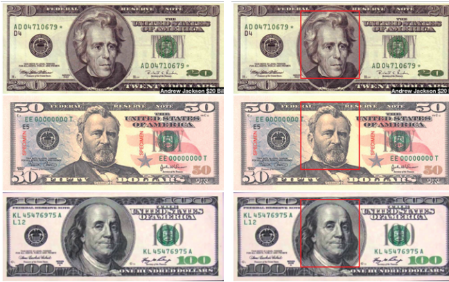
Figure 7.6 Result of the face-detection process. The right side has the images with the detected face surrounded by a box frame.
