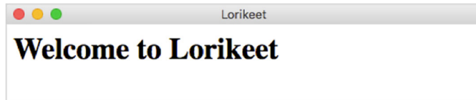
Figure 2.2 NW.js running a bare-minimum app. The app displays the contents of the index.html file, which means it's working as expected so far. Later in the chapter, you'll replace this simple HTML with the UI that makes up the app.
