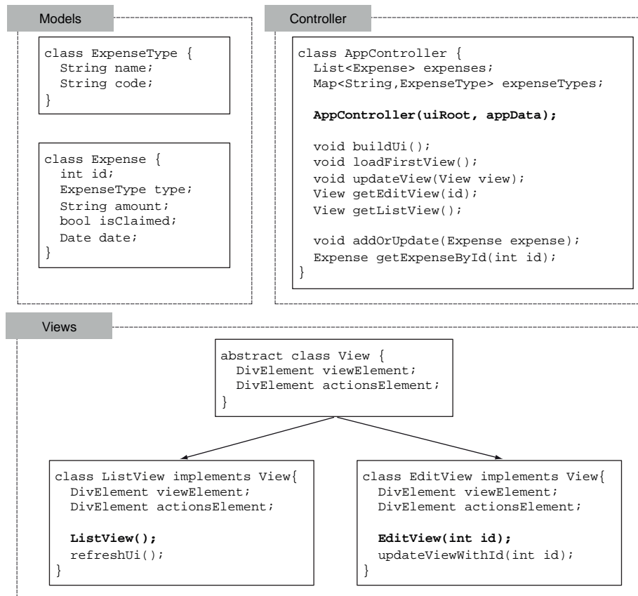
Figure 10.3 The main classes in the application are the models, the views, and the controller, with the constructors marked in bold.
