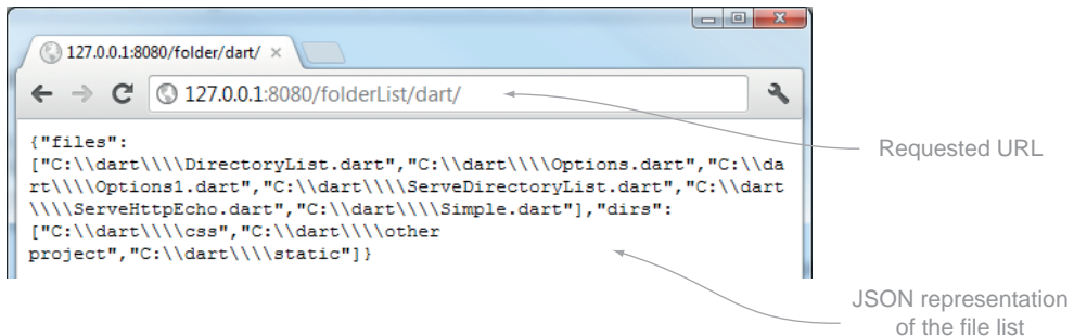
Figure 13.11 Returning JSON data from the server API
