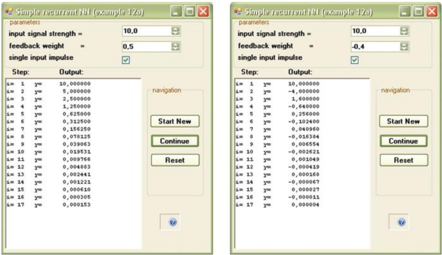
Figure 11.7 Stable progress of system with feedback after decreasing value of weight factor well below stabilization point.
