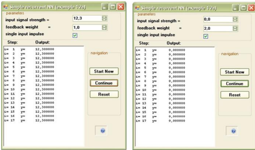
Figure 11.4 Two ways of achieving state of equilibrium in a linear network: zero signals (left) or single feedback amplification without simultaneous input signal (right).
