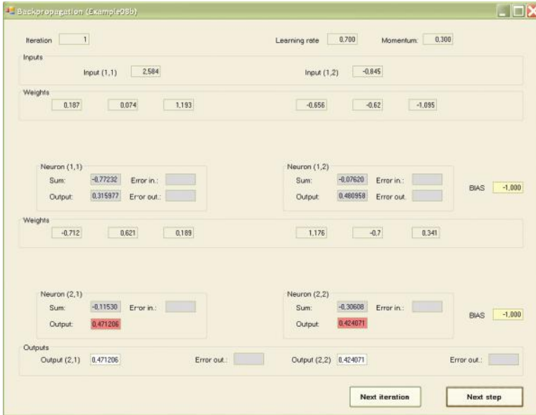
Figure 7.14 Network after finishing forward propagation.
