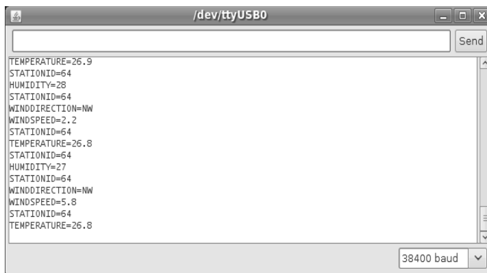
Figure 13-13. Weather Station Receiver values reported via the serial console
