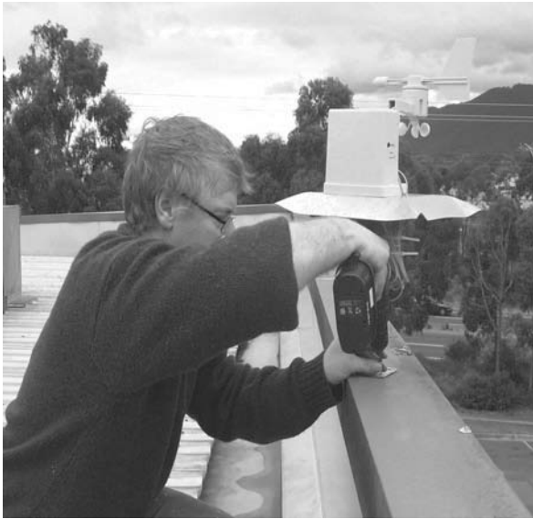
Figure 13-2. Weather station sensors and transmitter being installed
