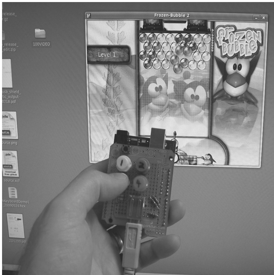
Figure 4-5. Using the virtual USB keyboard as a custom game controller
