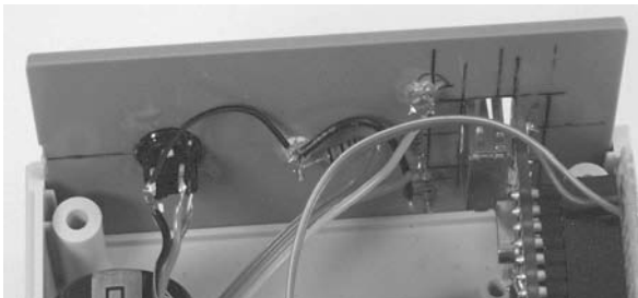
Figure 15-31. The Logging button and status LEDs glued into the front panel
