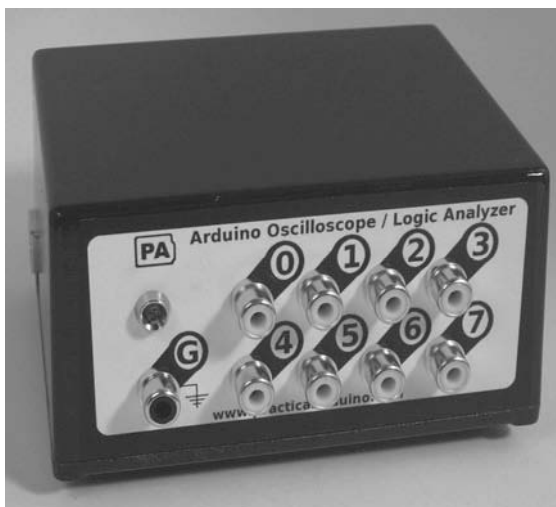
Figure 11-6. Connectors and LED mounted in front panel
