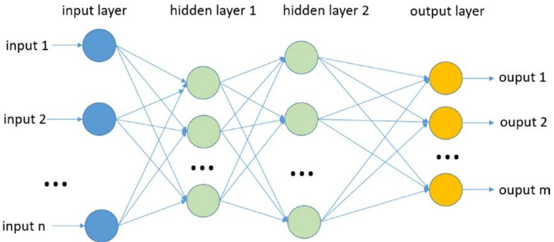
**Figure 9-6.** *The Multi Layer Perceptron (MLP) architecture*
