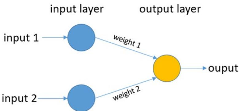
**Figure 9-3.** *The Single Layer Perceptron (SLP) architecture*
