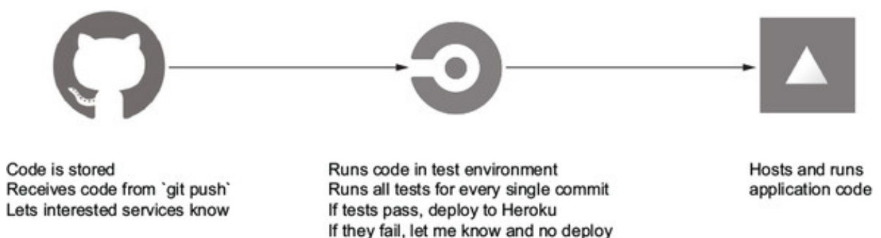
Figure 9.2. The Letters Social deploy pipeline. A CI build process is triggered when I (or anyone who contributes to the repository) push code. The CI provider (Circle, in this case) uses Docker containers to run your tests quickly and reliably. If the tests pass, the code will be deployed to whatever service you use to run your code. In our case, that's Now.
