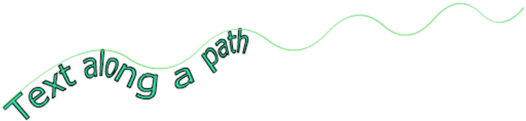
Figure 6-10. Text transformed along a path in the WarpingTextField3D example, using the TextField3D and PathAlignModifier classes
