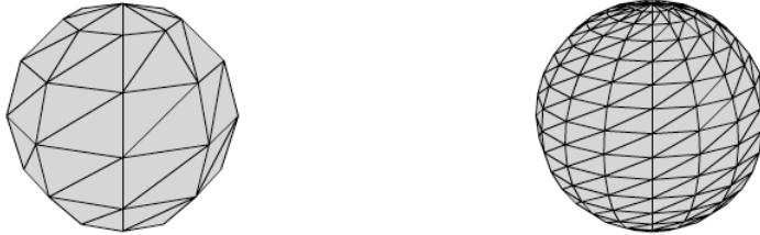
Figure 4-2. Default sphere (left) created with segmentsW = 8 , segmentsH = 6 , and sphere with higher level of detail (right), created with segmentsW = 24 , segmentsH = 12
