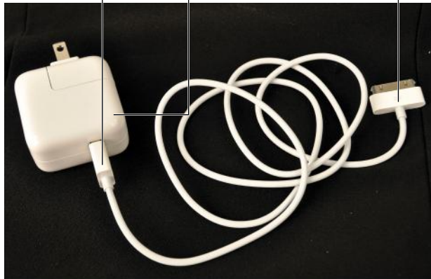
Figure 2-3: Assembling the connector cord and power adapter to charge the iPad battery.
