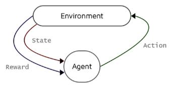
*Figure 17-1.* Basic flow of a RL algorithm. The agent observes the environment, executes an action to interact with the environment, and receives positive, negative, or zero reward.
