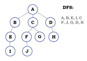
**Figure 15-5.** Traversing the tree using a DFS procedure; we begin at node A and then follow the path leading to the leftmost, non-visited node; therefore, we build the path formed by nodes A, B, E, I, then backtrack all the way up to the root (only node in the built path that has children pending discovery) and move to the leftmost, non-visited child, which would be C. It recursively executes the same procedure on C and eventually on node D, yielding the path seen on the graphic.
