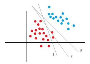
**Figure 11-5.** In the graphic, line number 1 incorrectly classifies two of the red points; therefore, we modify weights and bias to move it to the right a little bit; then classifying hyperplane 2 also makes a mistake classifying one of the red points. Finally, classifying hyperplane 3 makes no mistakes and properly divides red from blue points.
