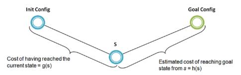
*Figure 15-11. Diagram showing the relation between G(s) and H(s)*
