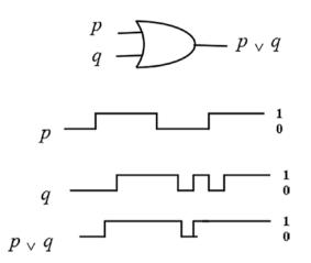
*Figure 1-3. Representation of disjunction component (OR)*
