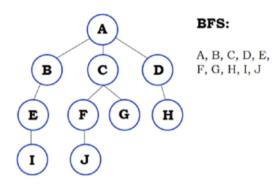
**Figure 15-4.** Traversing the tree using a BFS procedure; we begin at node A and then discover all nodes from the next level, i.e. nodes B, C, D. We continue like this, discovering nodes at the following level, i.e. nodes E, F, G, H. Finally, we discover nodes I and J at the final level.
