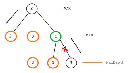
Figure 16-3. Pruning child nodes of MIN node with utility value 1
