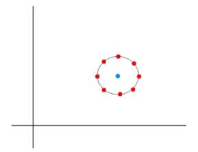
**Figure 14-3.** The neighborhood of the current solution (blue point) is formed by all the red points of the n-sphere surrounding it. In this case, n = 1; i.e., the 1-sphere is a circle.
