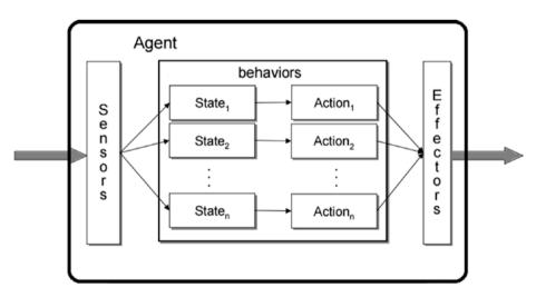
Figure 3-6. Reactive architecture diagram
