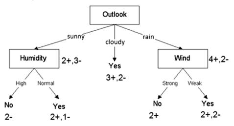
*Figure 10-6.* Validation set consisting of 16 training data classified by the DT. A positive number indicates a training data correctly classified by the DT, and a minus indicates an error in classification
