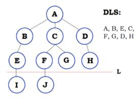
Figure 15-6. DLS is a DFS with an imposed depth limit L
