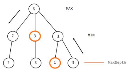
**Figure 16-2.** Execution of a Minimax algorithm where MaxDepth = 2. The method first calculates the values of nodes at MaxDepth and then moves those values up according to whether a node is a Max node or a Min node. Nodes denoted in orange are the ones selected to have their values elevated in the tree.
