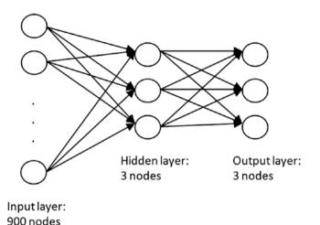
Figure 12-3. Structure of the proposed multi-layer NN
