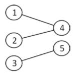
*Figure 11-2.* NN as a graph; neurons 4 and 5 are receiving inputs from neurons 1, 2, and 3, and neurons 1, 2, and 3 are having output connections to neurons 4 and 5.
