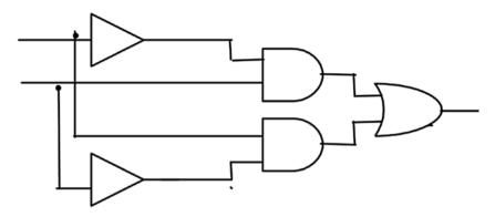
Figure 1-5. Binary comparer circuit
