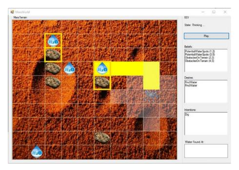
**Figure 4-5.** The rover creates a plan to go to location (3, 5), its closest probable water location, and so it creates a plan or sequence of actions (denoted in yellow cells) to get there and dig in.
