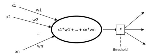
**Figure 11-3.** The Perceptron computes a weighted sum of the inputs and weights, submits this value to the activation function F, and transmits the signal to other neurons if and only if F turns out to be greater than or equal to a given threshold.
