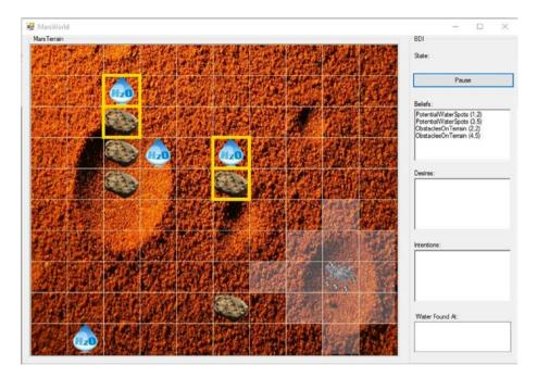
**Figure 4-4.** Windows Forms application showing the rover, its SenseRadius, beliefs of water locations and obstacles marked as yellow squares, and actual water and obstacle locations without any yellow square surrounding them
