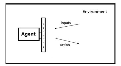
**Figure 3-1.** An agent in its environment. The agent uses its sensory components to receive inputs from the environment. It processes these inputs and eventually outputs an action that affects the environment. This will be a continuous interaction as long as the agent remains active.
