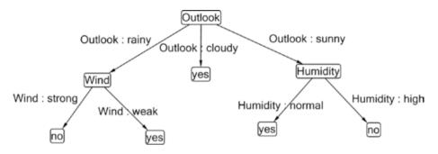
*Figure 10-2. Graphic of a DT matching the training data from Table 10-2 and created using MSAGL*
