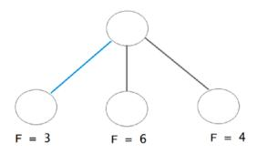
**Figure 15-10.** In a Best First Search method we always pick a node n with the lowest possible F(n) value to continue the search. In this case, F = 3, so the search continues from that node.
