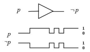
Figure 1-2. Representation of negation component (NOT)
