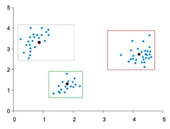
*Figure 13-6.* Centroids being recalculated as the average vector of the cluster they represent
