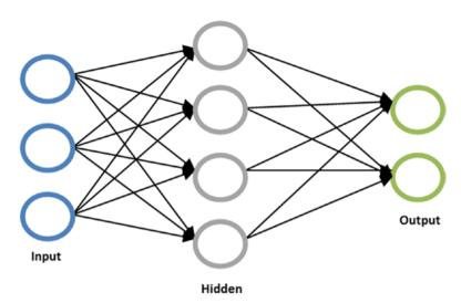
**Figure 11-11.** Multi-layer, feed-forward, fully connected NN consisting of three layers: one for input units, one for hidden units (gray) and one for output units (green). Sometimes the input layer is not considered as a layer.
