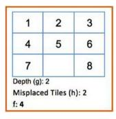
**Figure 15-12.** If we consider the blank tile, our path to a goal state would be 2, but in reality it is 1; thus, we are overestimating the real cost of a shortest path toward a goal state
