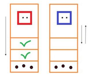
**Figure 3-4.** The cleaning agent (in blue) searches the environment, saving coordinates of visited cells, while the cleaning robot (in red) does not save the state of the environment or its history; therefore, it simply makes random moves that could take it up or down and even going in circles, thus consuming more time to clean the dirt on the last cell.
