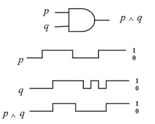
Figure 1-4. Representation of conjunction component (AND)
