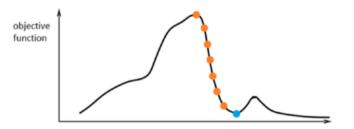
**Figure 14-2.** In this case, we minimize the objective function and go "downhill" through a path of orange points until we reach the blue point, a local minimum. We are minimizing, thus the blue point is a local minimum.
