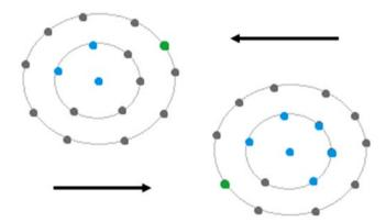
**Figure 15-8.** The forward search (on the left) and the backward search (on the right). The point in the middle indicates the current node being processed in the BFS, and the circles around it represent different levels of the tree. Blue points indicate nodes that have been discovered and processed during the search, and gray ones indicate queued nodes. The green points indicate the node where both searches would meet.
