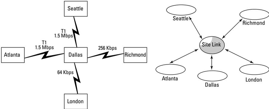
For the transport, in almost all cases, you should be using RPCs (also known within the AD tools as *IP transport*). Only use the alternative, SMTP, when RPCs aren't supported on the network link(s) between the sites (this is a relatively rare situation).
