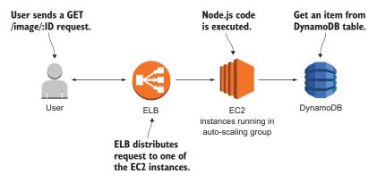
Figure 16.13 Looking up an image process in Imagery to return its state
