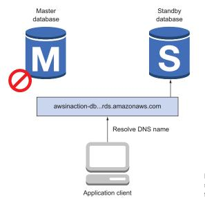
Figure 11.6 The client fails over to the standby database if the master database fails, using DNS resolution.
