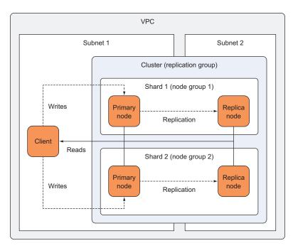
Figure 12.7 Redis deployment option: cluster with cluster mode enabled
