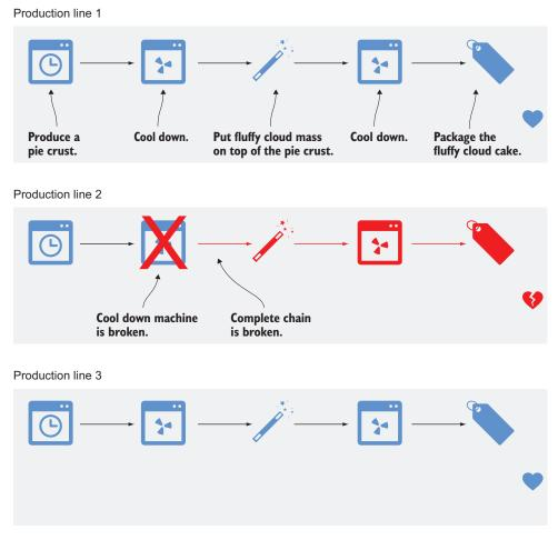
Figure 16.2 Redundancy eliminates single points of failure and makes the system more stable.
