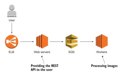
Figure 16.11 The Imagery application consists of two parts: the web servers and the workers.
