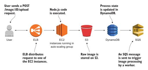
Figure 16.14 Uploading a raw image to Imagery and trigger image processing
