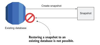
Figure 11.2 A snapshot can't be restored into an existing database.
