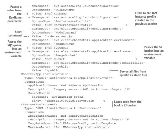
Under the hood, Elastic Beanstalk uses an ELB to distribute the traffic to the EC2 instances that are also managed by Elastic Beanstalk. You only need to worry about the configuration of Elastic Beanstalk and the code.
