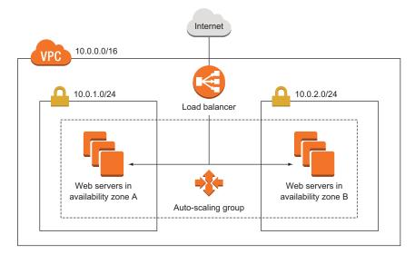
Figure 16.3 Fault-tolerant EC2 instances with an auto-scaling group and an Elastic Load Balancer
