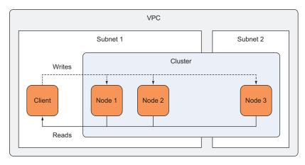
Figure 12.4 Memcached deployment option: cluster
