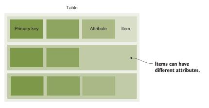
Figure 13.2 DynamoDB tables store items consisting of attributes identified by a primary key
