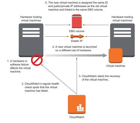
Figure 14.1 In the case of a hardware failure, CloudWatch triggers the recovery of the EC2 instance.
