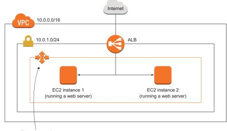
The auto-scalling group observes two EC2 instances. If a new EC2 instance is started, the auto-scaling group registers the EC2 instance with the ALB.
