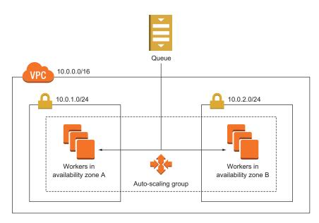
Figure 16.4 Fault-tolerant EC2 instances with an auto-scaling group and SQS
