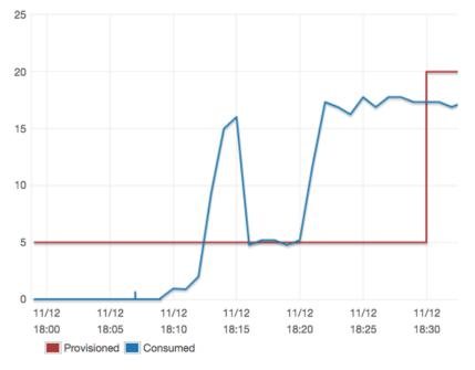
Figure 13.6 DynamoDB read capacity auto-scaling at work
