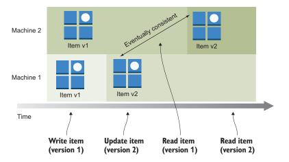
Figure 13.4 Eventually consistent reads can return old values after a write operation until the change is propagated to all machines.
