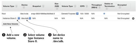
Figure 9.3 Adding an instance store volume manually
