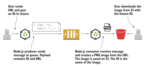
Figure 15.5 Node.js producer sends a message to the queue. The payload contains an ID and URL.
