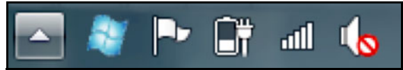
Figure 2.4 You can find the local cloud service icons in your notification area. The blue Windows flag tells you that the development fabric and the development storage services are running. Right-click the icon to show the UI you use to manage the services.
