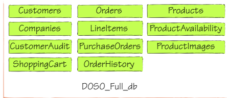
Figure 13.7 A sample application database schema for DayOldSushiOnline.com. The tables naturally fall into three families: customer data, orders and order history, and product data and pricing.
