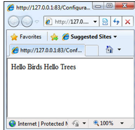
Figure 5.1 Displaying configuration settings in a web page. This text is being read from the appSettings section of the web.config file. Because you can't modify this text without redeploying your application, a better place to store it is in the ServiceDefinition.csdef file.
