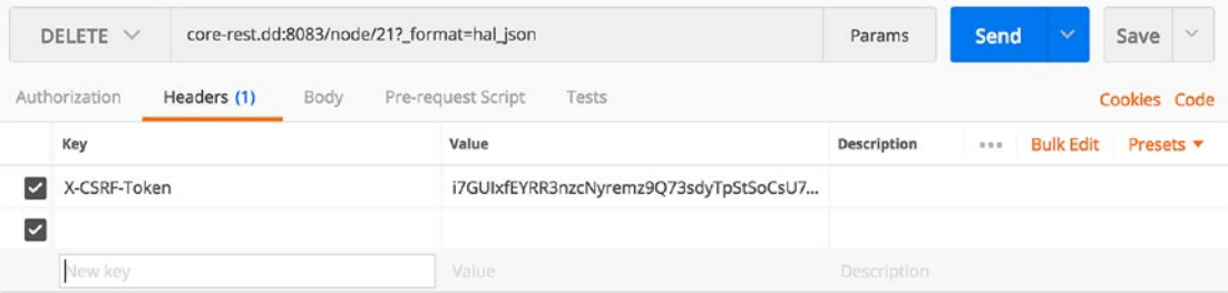
Figure 10-11. There is no need to designate a MIME type for our request body in a DELETE request, as it remains empty
