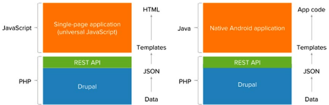
Figure 4-3. A decoupled Drupal implementation can serve any manner of Drupal-backed consumers, including a single-page application written in JavaScript (left) or a native mobile application written in Java for Android (right).
