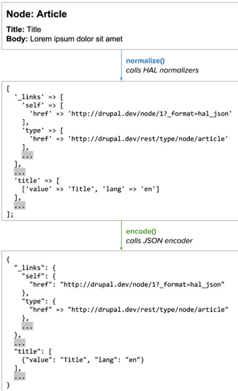
Figure 7-2. This diagram illustrates how normalization needs to occur before encoding to satisfy certain specifications like HAL, which dictate certain elements that should be part of the encoded format. In this example serialization, a node entity is normalized into a HAL-compatible structure before being encoded into the HAL+JSON format.
