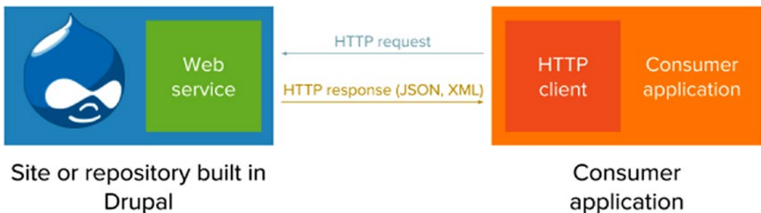
Figure 2-2. In this diagram, a Drupal site acting as a traditional site or content repository contains a web service (often a RESTful API) that accepts HTTP requests and issues HTTP responses in JSON or XML to an HTTP client located on a decoupled application, which might be server side or client side
