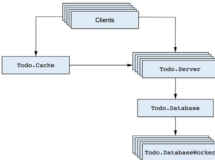
Figure 8.3 Processes in the to-do system
