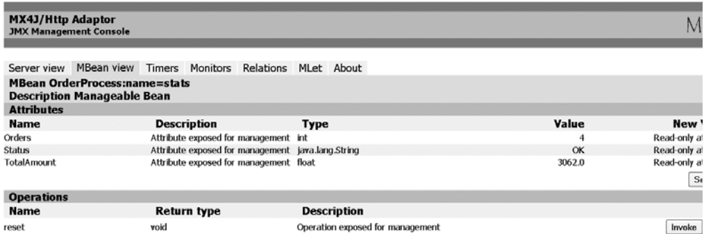
Figure 9-6. Invoking the reset method through the HTTP adaptor of MX4J
