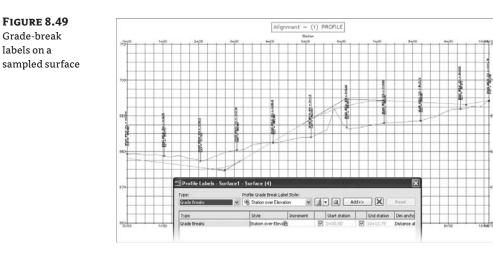
A sampled surface profile has grade breaks every time the alignment crosses a surface TIN line. Why wasn't your view coated with labels?
