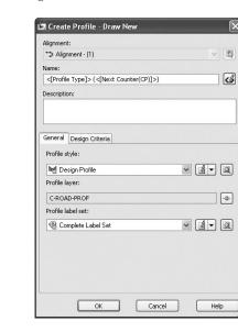
**4.** Click OK to accept the default settings. The Profile Layout Tools toolbar appears. Notice that the toolbar (see Figure 8.11) is *modeless*, meaning it stays open even if you do other AutoCAD operations such as Pan or Zoom.
