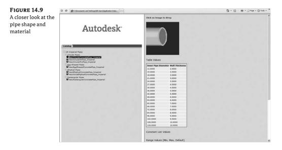
In this view, you can see the different inner pipe diameters and their corresponding wall thicknesses. Explore the other pipe shapes to get a feel for what is available.
