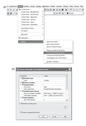
Occasionally, you'll receive AutoCAD point objects drawn at elevation from aerial topography information or other sources. It's also not uncommon to receive Softdesk point blocks from outside surveyors. Both of these can be converted to Civil 3D points under the Points > Utilities submenu or in the Create Points dialog (see Figure 4.8).
