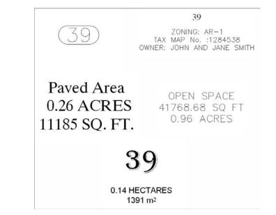
Parcel area labels are composed like all other labels in Civil 3D. You can select the following default parcel properties for text components of the label from the drop-down menu in the Properties selection box in the Text Component Editor dialog (see Figure 6.56):
