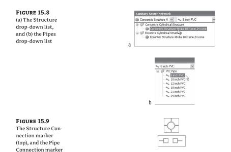
If you're placing parts and you'd like to connect to a pipe, hover over the pipe you'd like to connect to until you see a connection marker that has two square shapes. Clicking to connect to the pipe breaks the pipe in two pieces and places a structure (or null structure) at the break point.
