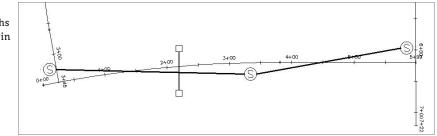
At least two potentially confusing elements show up in your profile view. First, the distance between structures (2D Length – Center To Center) isn't the same in plan and profile (see Figure 15.27) because the sanitary pipe doesn't run parallel to the alignment. Because the labeling reflects the network model, all labeling is true to the 2D Length – Center To Center or any other length you specify in your label style.
