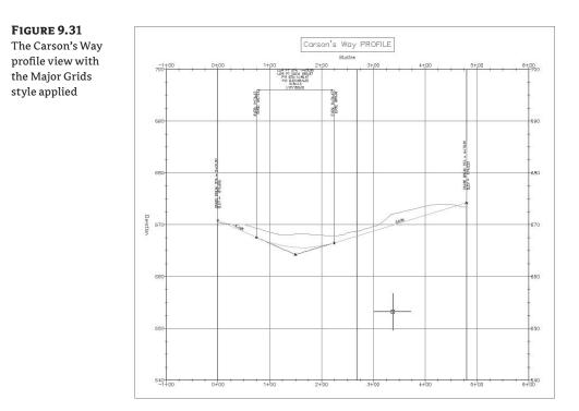
A profile view style includes information such as labeling on the axis, vertical scale factors, grid clipping, and component coloring. Using various styles lets you make changes to the view to meet requirements without changing any of the design information. Changing the style is a straightforward exercise, so next you look at what's happening behind the scenes when a profile view style is modified.
