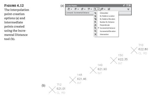
like to interpolate intermediate points every 25 feet. Instead of doing a manual slope calculation, you could use the Incremental Distance tool to create additional points (see Figure 4.12).
