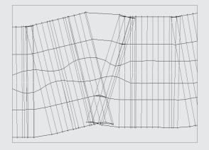
Bowties are problematic for several reasons. In essence, the corridor model has created two or more points at the same x and y locations with a different z, making it difficult to build surfaces, extract feature lines, create a boundary, and apply code-set styles that render or hatch.
