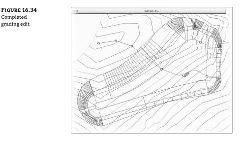
Editing any aspect of the grading will reflect instantly, and if other gradings within the group are dependent on the results of the modified grading, they will recalculate as well. Now that you have a working design, you can get a better view of the pond on the basis of stylizing the gradings, as described in the next section.
