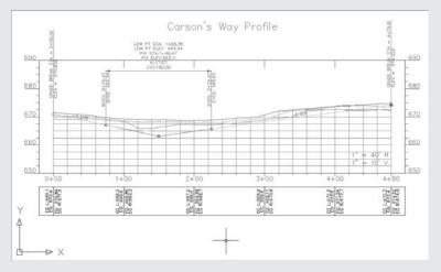
Band information can show any number of profiles, and by creatively using the offsets and profile assignments, you can apply labeling simply as well.
