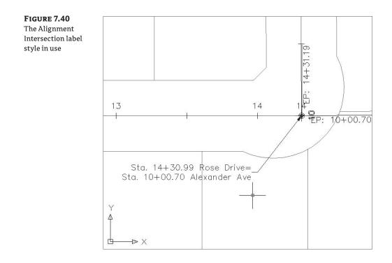
Thankfully, as you've already seen in the station offset label, you can access the properties of the alignment to generate a label. In this exercise, you'll use that same set of properties to create street-name labels that are applied and always up to date:
