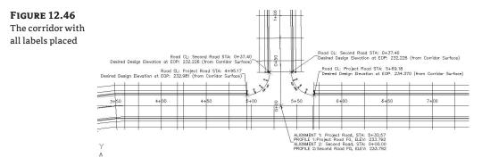
Now that you've added labels to the Start and End Stations of the EOP Right and EOP Left alignments, you can add labels to the EOP Right and Left FG profiles and then view the contours from the corridor surface:
