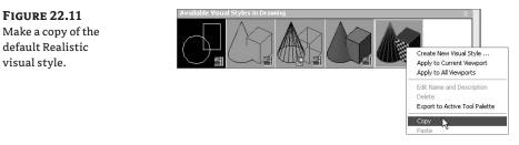
In your new visual style, change the Material Display toggle from Materials and Textures to Materials, and change the Edge Mode toggle from Isolines to None. You can rename your new visual style by right-clicking the style and choosing Edit Name and Description. Apply this customized visual style by right-clicking it and choosing Apply to Current Viewports. An example of this visual style is shown in Figure 22.12.
