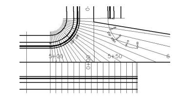
In the case of Figure 12.36, the first region of the EOP Left baseline was set to target the main road alignment instead of the secondary road alignment.
