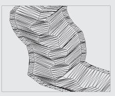
Another method for eliminating bowties is to notice the area where they seem to occur and adjust the regions. If your daylight links are overlapping, perhaps you can create an assembly that doesn't include daylighting and create a region to apply that new assembly.
