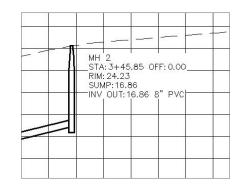
What if you wanted a profile-structure label with a line that could grow longer when you stretched it? If you go into the Label Composer for any structure label, you'll see two options for anchor points on the feature: Structure Dimension and Label Location. You can change and control the locations of both the Structure Dimension point and Label Location point.
