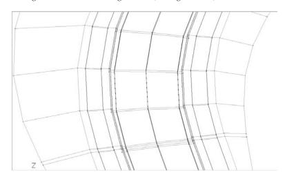
Corridor feature lines are similar to grading feature lines, which are studied in detail in Chapter 16. Both types of feature lines are stylized using Feature Line styles. Corridor feature lines can also be used as breaklines when a corridor surface is built, much like grading feature lines can be added to a surface as breaklines.
