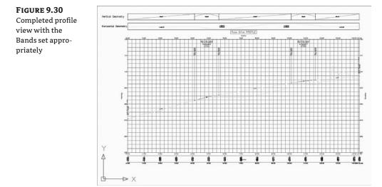
Bands use the Profile 1 and Profile 2 designation as part of their style construction. By changing what profile is referenced as Profile 1 or 2, you change the values that are calculated and displayed. These bands are just more items that are driven by styles, so the next section describes all the various styles in play with a profile view.
