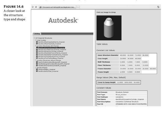
In this view, you can see the available sizes of the Concentric Cylindrical structure, such as 48″, 60″, 72″, and 96″. Follow the table to see what happens to the cone height, wall thickness, floor thickness, and frame diameter and height as the diameter dimension increases. The structure may get bigger or smaller, but its basic form remains the same and its behavior is predictable.
