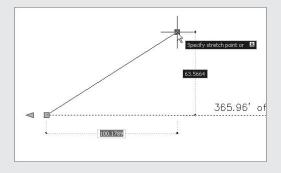
**Pipe Vertical Grip Edits in Profile** Using DYN in profile view lets you set exact invert, centerline, or top elevations without having to enter the Pipe Properties dialog or Prospector. Choose the appropriate grip, and note that the active DYN field is tracking profile elevation. Enter your desired elevation, and your pipe will move as you specify.
