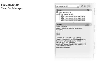
**11.** Double-click this sheet to open the new sheets drawing and display the layout tab for Haven CL 10+00.00 to 14+28.00. Review the multiple tabs created in this drawing file. The template used also takes advantage of AutoCAD fields, some of which don't have values assigned.
