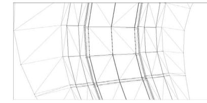
When building a surface from links, you have the option of checking a box in the Add as Breakline column. Checking this box will add the actual link lines themselves as additional breaklines to the surface. In most cases, especially in intersection design, checking this box forces better triangulation. It would be good practice to always check this box. If you find that you have an extremely large corridor and run into performance problems, consider leaving this box unchecked.
