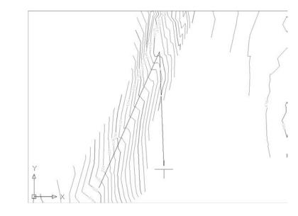
This second label indicates the average slope of a dirt road that is cut into the side of the site. By using a two-point label, you get a better understanding of the trend, as opposed to a specific point.
