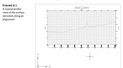
A profile is nothing more than a series of data pairs in a station, elevation format. There are basic curve and tangent components, but these are purely the mathematical basis for the paired data sets. In Civil 3D, you can generate profile information in one of the following three ways:
