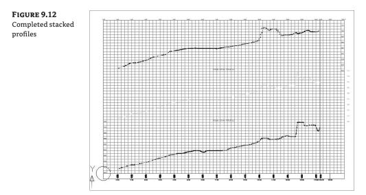
As you saw in Chapter 8, the styles for each profile can be adjusted, as can the styles for each profile view. The stacking here simply automates a process that many users found tedious. Once you have layout profiles created, they can also be added to these views by editing the Profile View Properties.
