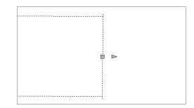
**FIGURE 15.17** Two types of pipe end grips A pipe midpoint also has two types of grips (see Figure 15.18). The first is a square location grip that lets you move the pipe using its midpoint as a basepoint. As before, you can take advantage of Stretch, Move, Rotate, and Scale by using your spacebar.
