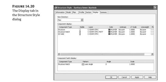
The display options for structure styles have a number of components that you need to review and understand. Use the View Direction pull-down menu to navigate between Plan, Model, Profile and Section components:
