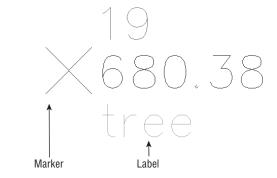
Point styles appear on the Settings tab of Toolspace under the Point branch (see Figure 4.21).
