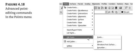
As noted earlier, you can create points from a surface elevation. But if you already have a batch of points in your drawing that you'd like to move up to a surface, you can use Points  $\geq$  Edit Points  $\geq$  Elevations from Surface (see Figure 4.19).
