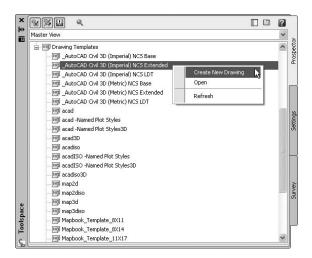
Civil 3D is built on both AutoCAD and Map, so Civil 3D 2009 comes with a variety of templates. However, most users will want to select one of the top few, which start with \_Autodesk Civil 3D and then have some descriptive text. These templates have been built on the basis of customer feedback to provide Civil 3D with a varying collection of object styles. These templates give you a good starting point for creating your own personal template file.
