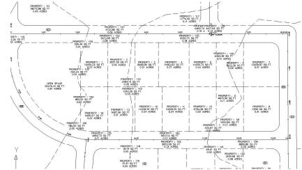
Another way to avoid site-geometry problems is to do site-specific tasks in different drawings and use a combination of external references and data references to share information.
