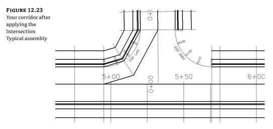
Your assembly has been applied; but because you haven't set the targets, the lane is only 12´ wide. You'll need to target the Second Road centerline from Station 0+00 through approximately Station 0+20 and the Project Road centerline from approximately Station 0+20 through 0+40:
