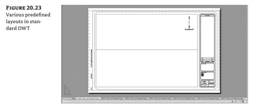
The viewports in these templates must be rectangular in shape and must have Viewport Type set to either Plan or Profile, depending on the intended use. You set Viewport Type on the Design tab of the Properties dialog, as shown in Figure 20.24.
