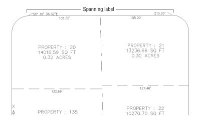
Spanning labels require that you use the appropriate vertices as discussed in detail in a previous section. Spanning labels have the following requirements:
