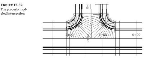
At this point, you have a properly modeled intersection, yet you haven't even begun the design. The next few sections will lead you through some techniques to assist you in refining the model and beginning the design process.
