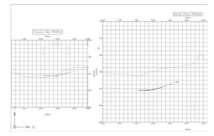
The target alignment is queried for an elevation at the intersecting station and a PVI is added to the superimposed profile. See Figure 9.15 for a bit of clarification. Note that this superimposed profile is still dynamic! A change in the Carson's Way layout profile will be reflected on the Parker Place profile view.
