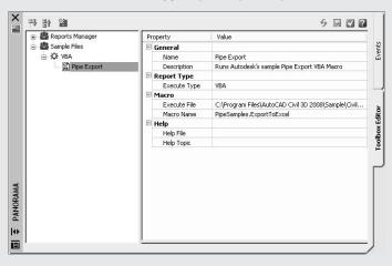
The text PipeSamples.ExportToExcel was determined by using the AutoCAD VBAMAN command to load up the same .dvb file, clicking the Macros button in that dialog, and copying the text from the Macro Name text field. The portion of the text that comes after the .dvb file extension in that text box is the macro name as required by the Toolbox Editor.
