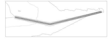
This corridor can be used to build a surface for a TIN-to-TIN volume calculation or can be used to create sections and generate material quantities, cross-sectional views, and anything else that can be done with a more traditional road corridor.
