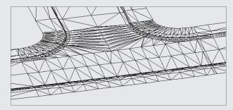
The resulting TIN occasionally needs more edge swapping than a corridor surface modeled with a complete set of links. Also keep in mind that because there are no links through part of the intersection, code-set styles designed for hatching and rendering may not work through the linkless region, and corridor-based material quantities may not be valid.
