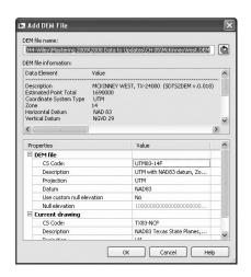
In addition to making a DEM a part of a TIN surface, you can build a surface directly from the DEM. The drawback to this is that no coordinate transformation is possible. Because one of the real benefits of using georectified data is pulling in information from differing coordinate systems, you're skipping this method to focus on the more flexible method shown here.
