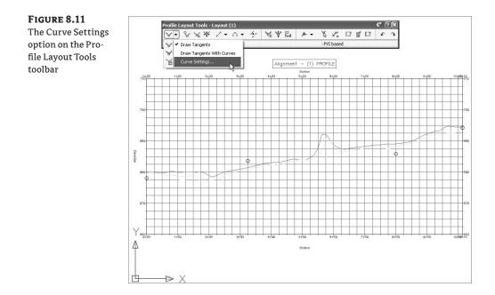
**6.** The Select Curve Type drop-down menu should be set to Parabolic, and the Length values in both the Crest Curves and Sag Curves areas should be 150.000'. Selecting a Circular or Asymmetric curve type activates the other options in this dialog.
