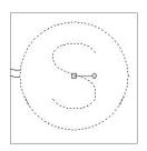
The second structure grip is a rotational grip that you can use to spin the structure about its insertion point. This is most useful for aligning eccentric structures, such as rectangular junction structures.
