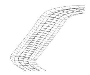
Choose Corridors ➤ Utilities ➤ Create Alignment from Corridor. Pick the corridor feature line that represents the swale on the right side of the centerline, as shown in Figure 12.3, to create an alignment.
