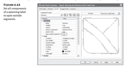
Spanning label styles must be composed to attach the desired spanning components (such as length and direction arrow) on the outside segment (as shown previously in Figure 6.63), with a small offset (see Figure 6.65).
