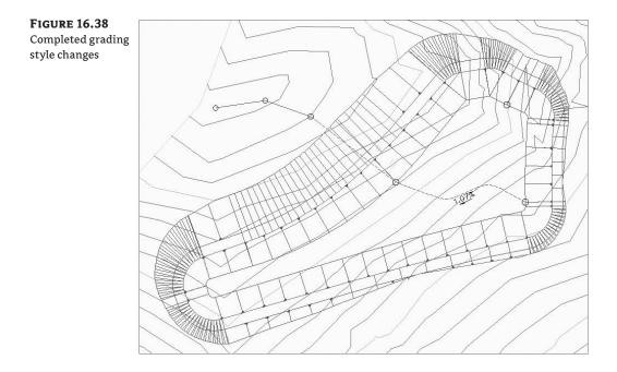
Although there are still some issues in the curve areas because of the way the gradings build feature lines, this view of your pond gives immediate feedback about the basic design. Note that the southeast corner contains slope arrows coming back to the pond area, indicating that the design is actually in a cut situation in this area. How much cut? You find out in the next section.
