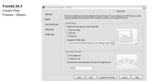
**Sheet Settings** In Civil 3D 2009, the Plan Production feature provides options for creating three types of sheets:
