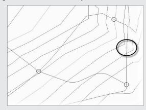
**39.** Enter **0.5**, → as the grade behind. A new elevation point will be created as shown here:
