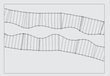
The TIN connected the points across the flat bottom and modeled the corridor perfectly, as you can see in the following image:
