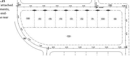
You can drag the diamond-shaped grip along the frontage to a new location, and the parcel segment will maintain its angle from the frontage. If the rear lot line is moved or erased, the attached parcel segments find a new endpoint (see Figure 6.22) at the next available parcel segment.
