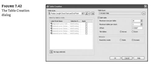
You can select a table style from the drop-down list or create a new one. Select a table layer by clicking the blue arrow. The selection area determines how the table is populated. All the label-style names for the selected type of component are presented, with a check box to the right of each one. Applying one of these styles enables the Selection Rule, which has the following two options:
