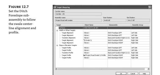
Click OK to dismiss the Target Mapping dialog. Click OK again to dismiss the Corridor Properties dialog and rebuild the corridor. The corridor should now look like Figure 12.8 when viewed in 3D.
