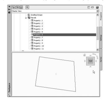
Within each drawing, the breakdown is similar. If a collection isn't empty, a plus sign appears next to it, as in a typical Windows Explorer interface. Selecting any of these top-level collection names displays a list of members in the preview area. Right-clicking the collection name allows you to select various commands that apply to all the members of that collection. For example, rightclicking the Point Groups collection brings up the menu shown in Figure 1.3.
