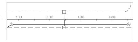
When pipes enter directly into profiled structures, they can be shown as ellipses through the Display tab of the Structure Style dialog (see Figure 15.36). See Chapter 14 for more information about creating structure styles.
