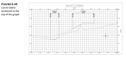
By using the top or bottom of the graph as the anchor point, you can apply consistent and easy labeling to the curve, regardless of the curve location or size.
