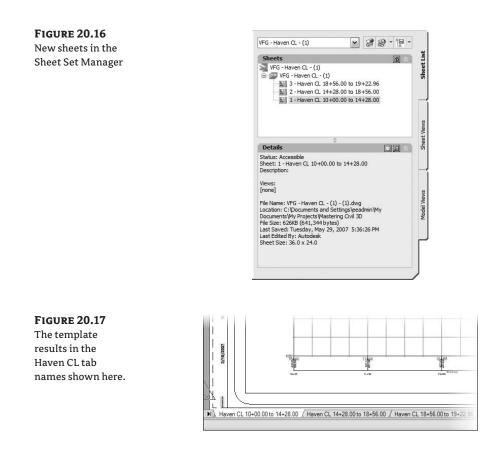
To create the final sheets in this new drawing, Civil 3D externally references (XRefs) the drawing containing the view frames; creates data references (DRefs) for the alignments, profiles, and any additional objects you selected in the Create Sheets Wizard; and, if profile-sheet types were selected in the wizard, creates profile views in the final sheet drawing.
