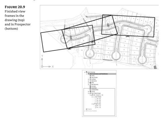
The numbering for your view frames, view-frame groups, and match lines may not identically match that shown in the images. This is due to the incremental counting Civil 3D performs in the background. Each time you create one of these objects, the counter increments. You can reset the counter by modifying the name template.
