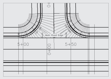
You can use similar techniques to model additional design elements such as left-turn lanes, widening, asymmetrical intersections, and interchanges. The best way to tackle an intersection is to sketch the intersection layout and figure out how the components are related. Map out baselines, regions, targets, and subassemblies. Once you have a plan for your intersection, build all the required pieces and use the corridor to join your model together.
