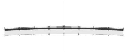
Note that the LaneParabolic subassembly doesn't have a Side parameter. The parabolic nature of the component results in a single attachment point that would typically be the assembly center-line marker.
