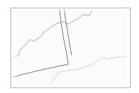
**15.** Click the Edit Curve tool on the Feature Lines toolbar, and pick Feature Line B to display the Edit Feature Line Curve dialog shown in Figure 16.17.
