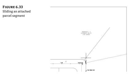
**11.** Notice when you place the parcel segment at a new location that the segment endpoint snaps back to the rear parcel segment (see Figure 6.34). This is typical behavior for an attached parcel segment.
