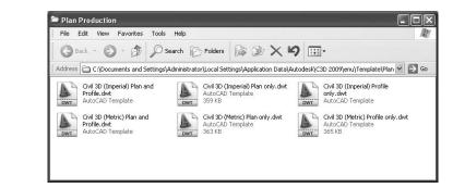
Each template contains layout tabs with pages set to various sheet sizes and plan scales. For example, the Civil 3D (Imperial) Plan and Profile.dwt template has layouts created at various ANSI and ARCH sheets sizes and scales, as shown in Figure 20.23.
