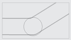
If inside or outside walls (or both) are shown when a pipe is drawn in plan view, there is an option that allows for cleanup at pipe connections.
