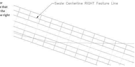
**3.** In the Create Alignment dialog, name the alignment **Swale CL**. Keep the default values for the Style and Label options, and deselect the Create Profile check box. You'll add the profile another way. Click OK to dismiss the dialog, and notice that an alignment has been created at the corridor feature line (see Figure 12.4).
