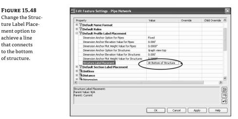
Changing the feature settings requires you to reset the label, but once you replace the label you should see the line go all the way to the bottom of the structure.
