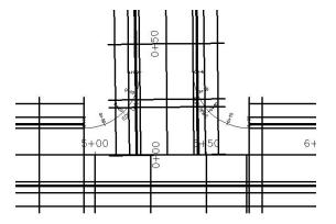
Notice that the region for the second baseline extends all the way to the end of the Second Road alignment. You must now adjust this to match the EOP points of curvature:
