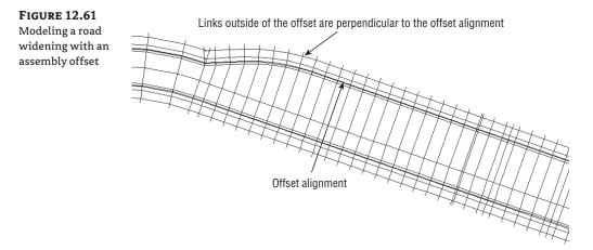
Typical examples of when you'll use an assembly offset include transitioning ditches, widening roads, traffic-calming lanes, interchanges, and other applications. The assembly in Figure 12.62, for example, includes two assembly offsets. The assembly could be used for transitioning roadside swales, similar to the first exercise in this chapter.
