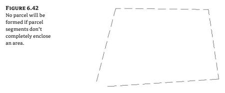
There are times in surveying and engineering when parcels of land don't necessarily close when created from legal descriptions. In this case, you must work with your surveyor to perform an adjustment or find some other solution to create a closed polygon.
