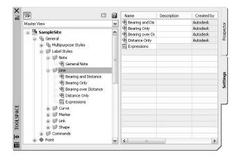
Because building label styles is a critical part of producing plans with Civil 3D, a later section of this chapter looks at how to build a new basic label and some of the common components that appear in every label style throughout the product.
