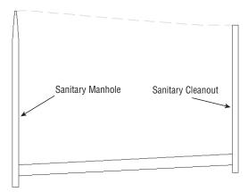
**Recommended Pipes:** 8", 10", 12" PVC pipe per manufacturer dimensions.
