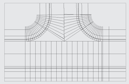
The resulting corridor surface uses the principles explained in the section "Building a First Draft Corridor Surface" in Chapter 11 to create the TIN, and therefore corridor points are connected to complete the lanes with TIN lines. The next image clearly shows the triangulation along the crowned section and no gaps anywhere in the intersection:
