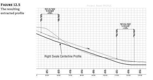
**6.** Pan over to your newly extracted swale centerline alignment. Add a PI around Station 13+00 in plan. You can use the transparent commands to snap the PI to Station 13+00 exactly or place it approximately at Station 13+00.
