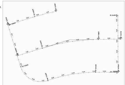
Each of these alignments is simply a pointer back to the original file. They can be stylized, stationed, or labeled, but the definition of the alignment cannot be changed. This is more clearly illustrated in a surface, so add a surface reference now:
