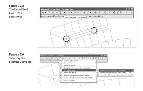
**7.** Ctrl-click the fixed-line segment you drew in steps 4 and 5. A blue rubber band should appear, indicating that the alignment of the curve segment is being floated off the endpoint of the fixed segment (see Figure 7.10). The Ctrl-click is required to make the pick activate the alignment segment and not the polyline entity.
