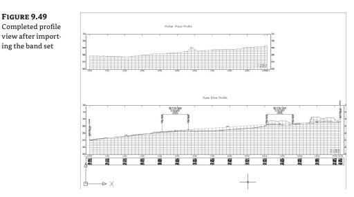
Your Rose Drive profile view now looks like the Carson's Way profile view. Band sets allows you to create uniform labeling and callout information across a variety of profile views. By using a band set, you can apply myriad settings and styles that you've assigned to a single profile view to a number of profile views. The simplicity of enforcing standard profile view labels and styles makes using profiles and profile views simpler than ever.
