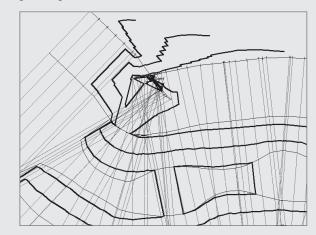
When your corridor surface is created, the TIN has to make some assumptions about crossing breaklines that can lead to strange triangulation and incoherent contours, such as in the following graphic:
