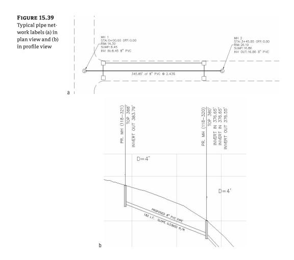
Like all Civil 3D objects, the Pipe and Structure label styles can be found in the Pipe and Structure branches of the Settings tab in Toolspace.
