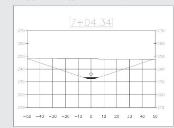
The following exercise will lead you through building a pipe trench corridor based on an alignment and profile that follow a pipe run, and a typical trench assembly.
