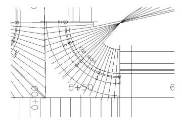
Fix this problem by reversing your alignment direction and rebuilding the corridor, or editing your subassembly to swap the lane to the other side of the assembly. If you want to minimize the number of assemblies in your drawing, note which directions the intersection alignments should run to accommodate one intersection assembly.
