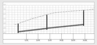
Notice how the slope remains constant even as the pipe cover increases. Maximum cover is a *violation only* rule, which means it never forces a pipe to increase slope to remain within tolerance; it only provides a warning that maximum cover has been violated.
