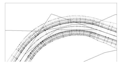
**Typical Cause** You accidentally chose the Existing Ground profile instead of the Finished Ground profile for your baseline profile. Most corridors are set up to sample at every vertical geometry point, and a sampled profile, such as the Existing Ground profile, has many more vertical geometry points than a layout profile (in this case, the Finished Ground profile). These additional points on the Existing Ground profile cause the unexpected sample lines and flags that something is wrong.
