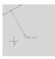
While the command is active, you can toggle between angle, bearing, deflection, and azimuth by following the command-line prompts.
