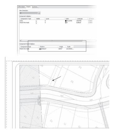
You define the match-line style in the drawing containing the view frames. Any changes to the style must be made in the view-frames drawing; the drawing must then be saved and the XRef updated in the sheets drawings. If you created the layout sheets in the drawing in which the view frames exist, the match-line style updates are automatically displayed on the layout sheets.
