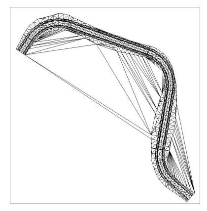
**FIGURE 11.33** A corridor surface after the addition of an automatic daylight boundary
