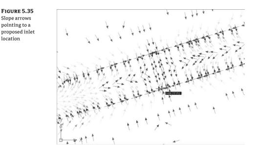
With these simple analysis tools, you can show a client the areas of their site that meet their constraints. Visually strong and simple to produce, this is the kind of information that a 3D model makes available. Beyond the basic information that can be represented in a single surface, Civil 3D also contains a number of tools for comparing surfaces. You compare this existing ground surface to a proposed grading plan in the next section.
