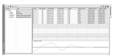
This interface allows you to optimize your best fit by adding more points, selecting the check box in the Pass Through column to force one of your points on the line, or adjusting the value under the Weight column. Figure 2.28 shows the a line drawn by best fit.
