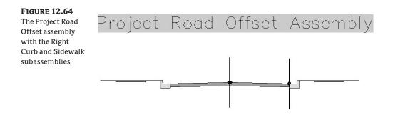
Now that the assembly is built, you need a profile representing EOP before you can adjust the corridor model. You have several options for creating this profile, such as using Profiles  $\geq$  Create by Layout or any other valid profile-creation technique. In this case, the corridor surface in this drawing can provide a valid profile for your offset:
