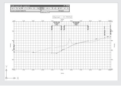
5. Set Elevation Change to 4.000<sup>°</sup>. Click the Station Range radio button, and set the Start value to 0+ 10<sup>°</sup> and the End value to 8+50.00<sup>°</sup>. You're moving the internal PVIs 4<sup>°</sup> vertically while maintaining the endpoints of the design. Click OK.
