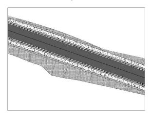
A code set style can be created to enhance your corridor's appearance for things like exhibits at public hearings. Instead of spending time creating a series of hatch boundaries using polylines and then manually applying hatches to areas of paving, sidewalks, curbs, and so on, you can have the code set style automatically hatch those areas for you.
