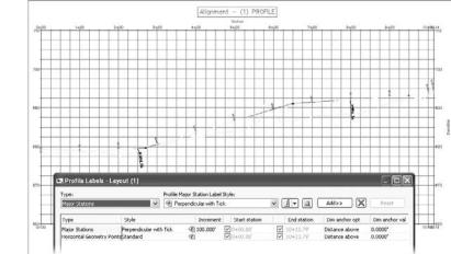
**10.** In the middle of the Profile Labels dialog, change the Increment value in the Major Stations row to 50, as shown in Figure 8.41. This modifies the labeling increment only, not the grid or other values.
