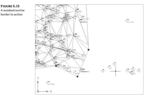
Notice how the triangulation appears to include lines to nowhere. This is the nature of the nondestructive breakline. The points you attempted to exclude from the surface are still being included in the calculation; they are just excluded from the display. This isn't the result you were after, so fix it now:
