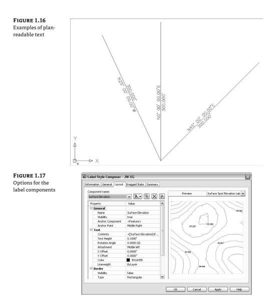
Labels are made of individual components. A component can be text, a block, or a line, and the top row of buttons controls the selection, creation, and deletion of these components:
