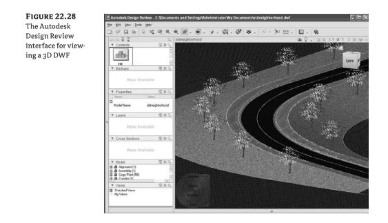
The navigation tools in the Design Review environment are identical to those in an AutoCADbased interface, such as 3D orbit, pan, and zoom.
