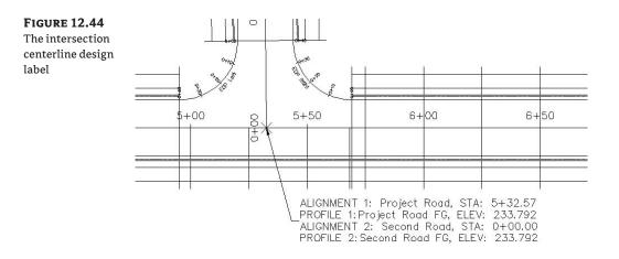
Note that the elevations of the Project Road FG and Second Road FG are both equal to 233.792. If the label indicated that these elevations weren't the same, you would need to edit your profile geometry to make sure they matched. This label will be useful during later stages of the design process. As you iterate your FG profiles, this label will alert you to any adjustments that are required to make the profiles match at their intersection.
