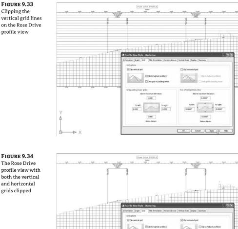
FIGURE 9.34 The Rose Drive profile view with both the vertical and horizontal grids clipped
