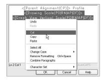
The Drawing Scale and the Graph View Vertical Scale properties, which were cut from the preview screen in step 10, aren't available for selection in the axis labels, only in the title label. But the program understands the field codes you just cut and will let you use them in the axis labels by pasting them in, even if they can't be selected directly. (This is one of our favorite hacks for getting around the limitations that are in Civil 3D!)
