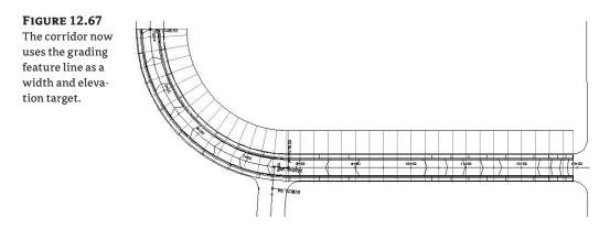
Once you've linked the corridor to this feature line, any edits to this feature line will be incorporated into the corridor model. You can establish this feature line at the beginning of the project and then make horizontal edits and elevation changes to perfect your design. The next few steps will lead you through making some changes to this feature line and then rebuilding the corridor to see the adjustments.
