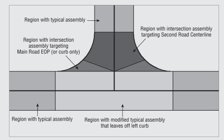
Instead of a right-lane-only assembly, you need an assembly that is fundamentally the typical road section minus the left curb, sidewalk, and so on, as in the following graphic.
