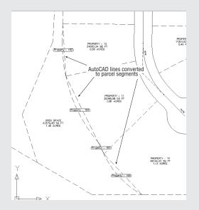
• Use line segments and the Create Parcel from Objects menu command for final detailed segment work. Surveyors often prefer to lay out straight-line segments rather than curves, so for the final rear-lot line cleanup, create AutoCAD lines across the back of each lot and then use Create Parcel from Objects to turn those lines into parcel segments, as shown here:
