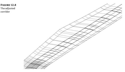
Note that the corridor has been adjusted to reflect the new target alignment and profile. Also note that you may want to increase the sampling frequency. You can view the sections using the View/Edit Corridor Section tools. You can also view the corridor in 3D by picking it, right-clicking, and choosing Object Viewer. Use the 3D orbit tools to change your view of the corridor.
