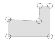
Corridors built using the BasicCurbandGutter subassembly are most commonly used for building top and datum surfaces, rendering curb-and-gutter areas, and creating cross sections. The BasicCurbandGutter subassembly can return quantities of concrete (or other curb-and-gutter construction material) but not gravel bedding or other advanced material layers.
