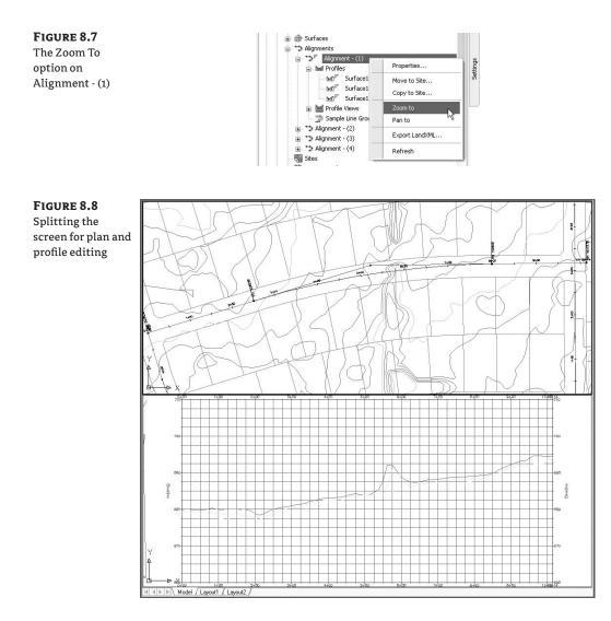
By maintaining the relationships between the alignment, the surface, the sampled information, and the offsets, Civil 3D creates a much more dynamic feedback system for designers. This can be useful when you're analyzing a situation with a number of possible solutions, where the surface information will be a deciding factor in the final location of the alignment. Once you've selected a location, you can use this profile view to create a vertical design, as you'll see in the next section.
