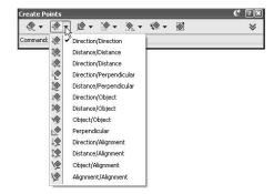
**Alignment Point-Creation Options** The options in the Alignment category are designed for creating stakeout points based on a road centerline or other alignments. You can also set Profile Geometry points along the alignment using a tool from this menu. See Figure 4.10.
