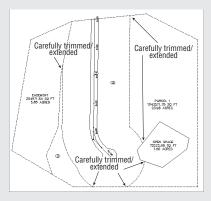
• Use the Create Parcel by Layout menu command with the attached segment tools for internal parcels. The precise sizing tools and Free Form Create automatically create only one attached segment between parcels, so using them to create your subdivision lot boundaries ensures proper parcel geometry, as seen in Properties 1 through 19 in this graphic:
