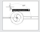
Press your down arrow key to get a shortcut menu that allows you to specify a basepoint followed by a rotation angle, as well as options for Copy and Undo. DYN combined with the Rotate command is beneficial when you're rotating eccentric structures for proper alignment.
