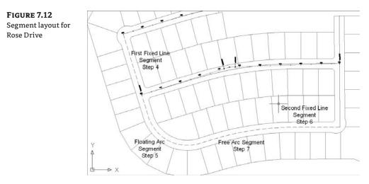
**6.** Return to the toolbar, and select the Draw Fixed Line (Two Points) tool again. Draw the line on the east end of this proposed street. This segment is still be part of the alignment, in spite of not being connected!
