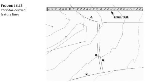
**4.** Using an Endpoint osnap, pick the end point on A just to the northwest of Feature Line B. Using an Endpoint osnap, pick the next end point on A to the east, leaving a gap, as shown in Figure 16.14.
