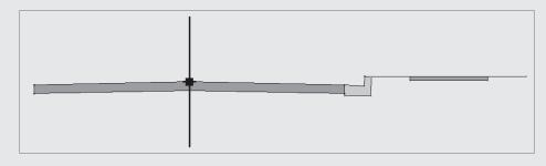
You can use the same intersection assembly for the EOP baselines as in the exercise, but the region that would normally target the Main Road centerline now targets an alignment and corresponding profile that follows the edge of the Main Road left lane. The following graphic shows the location of this target alignment:
