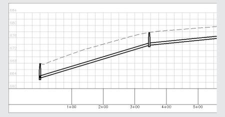
When you start from the downhill side of your project, the Minimum Slope Rule is applied as long as minimum cover is achieved. The following graphic shows a pipe run that was created starting from the downstream location (left to right):
