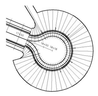
You can fix this problem by reversing your alignment direction and rebuilding the corridor or editing your subassembly to swap the lane to the other side of the assembly.
