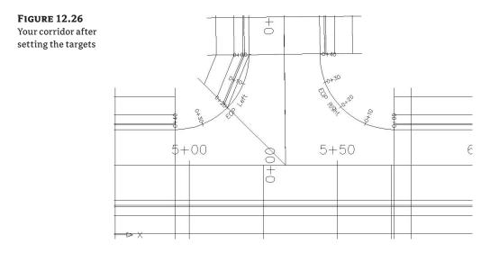
The target is set correctly for your first region, but the sampling frequency of the corridor is too far apart, resulting in a chunky appearance. You'll now adjust the sampling frequency:
