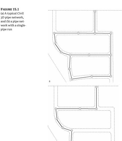
*Null structures* are created automatically when two pipes are joined together without a structure; they act as a placeholder for a pipe endpoint. They have special properties, such as allowing pipe cleanup at pipe intersections. Most of the time, you'll create a style for them that doesn't plot or is invisible for plotting purposes.
