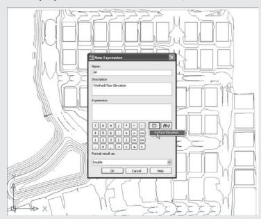
6. Click the Insert Property button and select Surface Elevation, as shown here.
