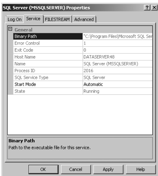
FIGURE 3-2 Use Service tab options for setting the start mode.
