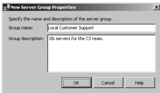
FIGURE 5-4 Enter a name and description in the New Server Group Properties dialog box.
