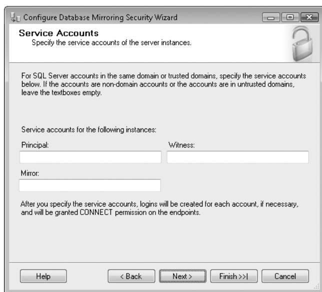
FIGURE 17-9 Configure service accounts in the same or trusted domains.
