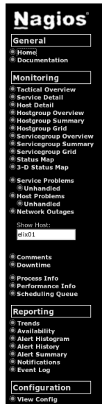
Figure 16.1: The subitem Unhandled under both the Service Problems and Host Problems menu items has only been on the start page of the Nagios Web interface since Nagios 3.0.
