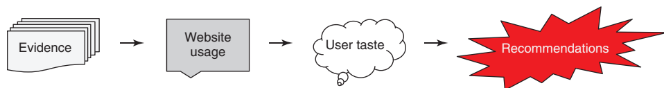
Figure 3.1 Data flow from evidence to recommendations. You start with your evidence, which you can aggregate into website usage. With that, you can start to understand the user's tastes, which can work as input to the recommender system to produce recommendations.
