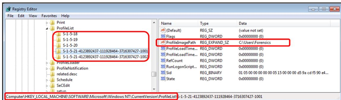
Figure 6: The list of system profiles
