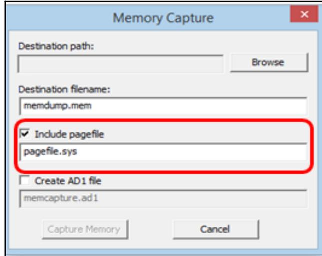
Figure 1: FTK imager; adding page files during memory acquisition
