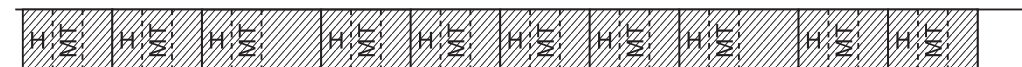
Figure 9-1. A fragment of the Managed Heap (inside Small Object Heap) right at the beginning of the GC process (H stands for header, MT stands for method table pointer, objects are marked by light gray filling)
