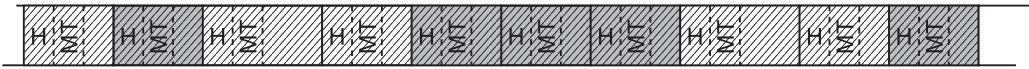
Figure 9-2. A fragment of the Managed Heap right after Mark phase (medium gray objects are marked)
