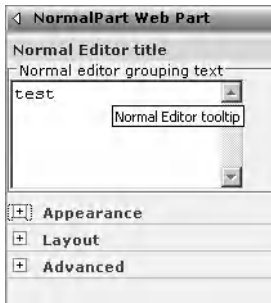
Figure 1-14. Adding a custom control to the web part editor tool pane
