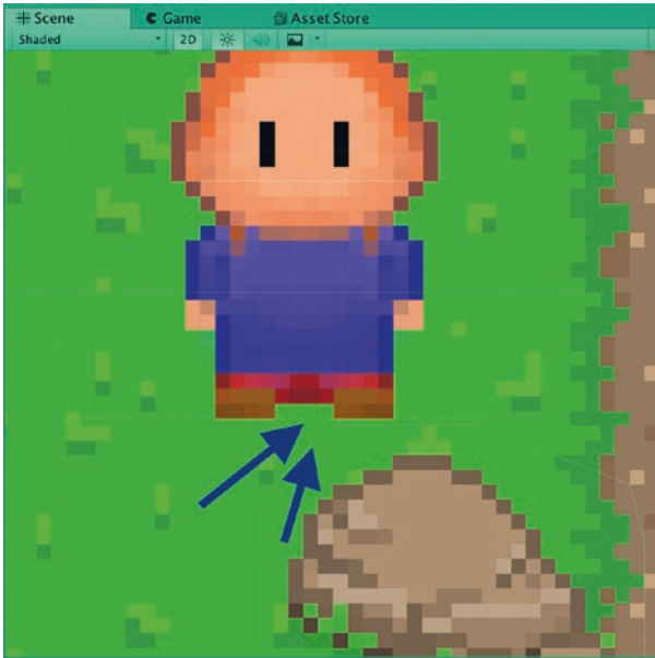
Figure 4-33. The gap between the Player and objects around her are due to the collider boxes—the thin green box
