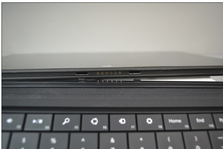
Figure 2-7: Match the Touch or Type keyboard's connector with the connector on the bottom of your Surface, and they click into place.
