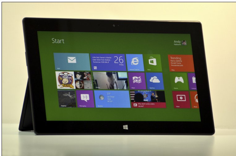
Figure 1-1: The Surface includes a kickstand to prop it up at a comfortable viewing angle.
