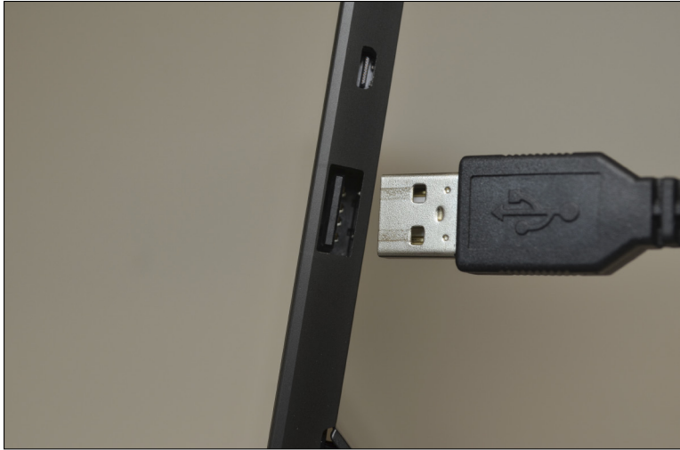
Figure 6-11: Plug the large end of your camera's cable into your Surface's USB port, located on the right side.
