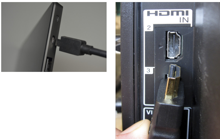
Figure 6-14: Both ends of the microHDMI cable used to connect a Surface with Windows RT to a monitor.
