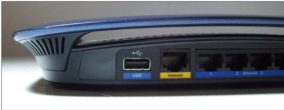
**Figure 7-8:** A USB port on a router for an external storage device.
