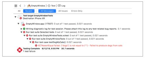
Figure 9-13. The Report navigator describes a test failure
