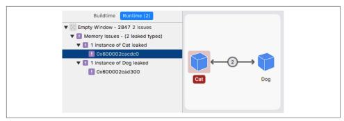
Figure 9-25. The memory graph displays a leak
