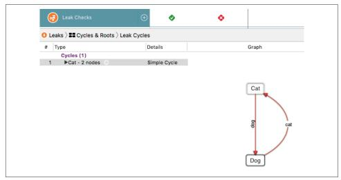
Figure 9-27. Instruments describes a retain cycle
