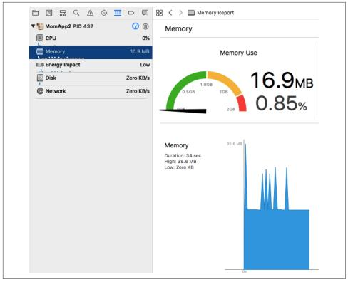
Figure 9-23. The Debug gauges
