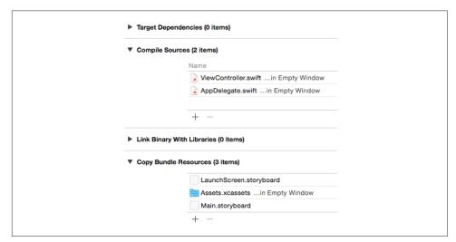
Figure 6-8. The app target's build phases
