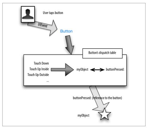
*Figure 11-1. The target–action architecture*
