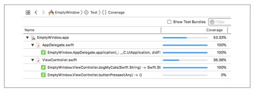
Figure 9-14. The Report navigator displays code coverage statistics
