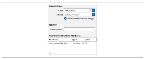
Figure 7-18. Rounding a button's corners with a runtime attribute
