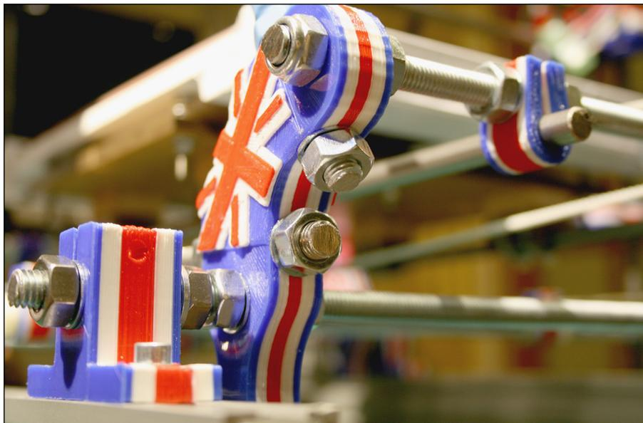
**FIGURE 14-18:** Layer-selective color printing with a single extruder involves using different layer heights.
