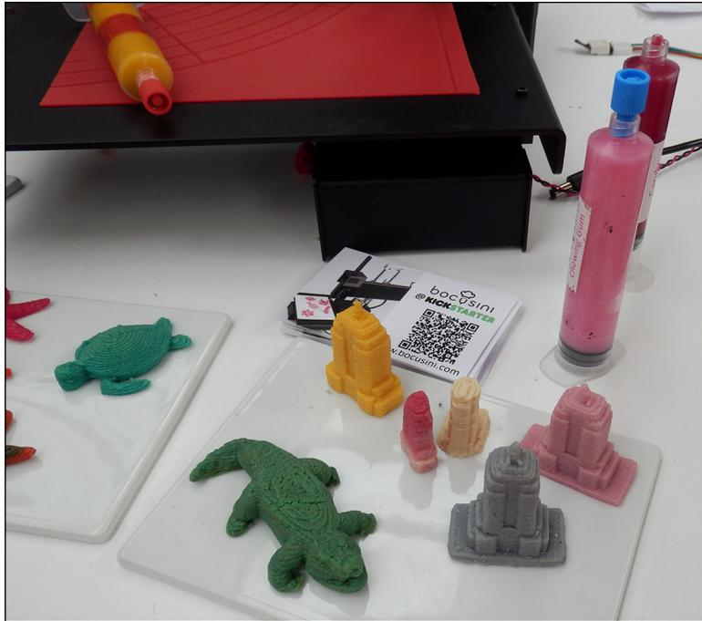
**FIGURE 10-16:** Some 3D printers use filled tubes or syringes of flavored pastes to print fun, edible shapes.
