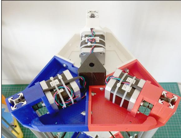
Because the printer is mainly 3D-printed and able to print its own parts, the 3DR delta printer is easy to change, evolve, or even scale up or down in whatever way you require.
