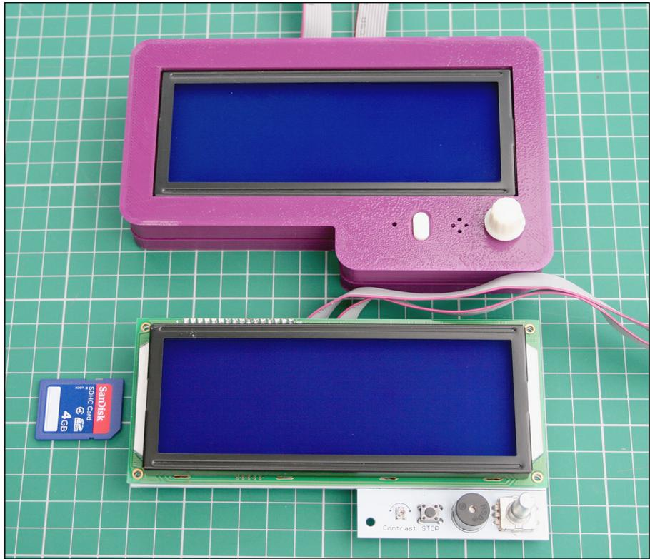
**FIGURE 13-9:** A bare electronics display board (bottom) and the same board housed in a 3D-printed enclosure (top).
