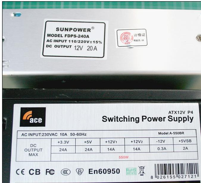
**FIGURE 13-14:** Power information on a power supply.
