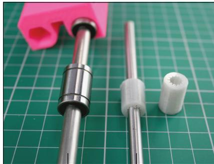
**FIGURE 12-5:** The rods and bearings used in a 3D printer allow the carriage or axis to slide smoothly along or up and down.
