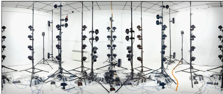
**FIGURE 5-12:** Photogrammetric studio using 110 Canon DSLR cameras synchronized by six laptop computers.
