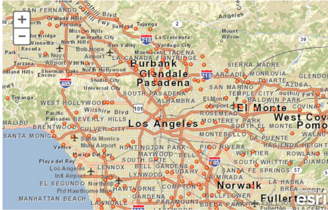
Figure 2.13 FeatureLayer with DefinitionExpression of 'TOTAL_POP > 5000' applied
