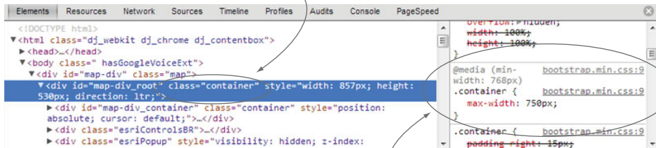
Figure 4.20 Chrome debug console to debug style sheet conflicts
