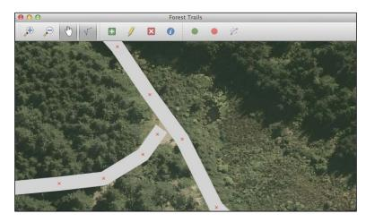
The tracks aren't connected together. Since the user can click anywhere on the map, there's no way of ensuring that the tracks are connected — and if the tracks aren't connected, the **Find Shortest Path** command won't work.
