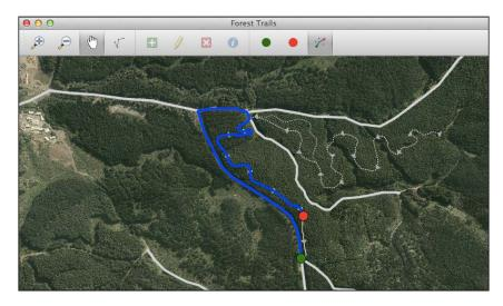
If you look carefully at the preceding screenshot, you'll see that the path taken wasn't the shortest one; the starting point was at the bottom and the ending point was near the end of a one-way bike track, so the shortest available path involved taking the road back to the start of the one-way track, and then following it through to the endpoint. This is exactly the behavior that we would expect, and it is correct given the one-way nature of the tracks.
