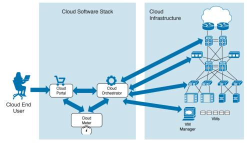
Figure 4-1 Cloud Computing Architecture
