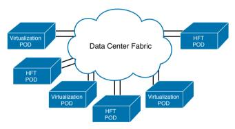
Figure 14-3 Data Center Logical Scaling Model
