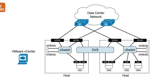
Figure 6-5 Comparing a VMware vSwitch and a VMware DVS
