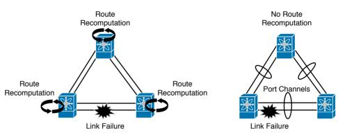
Figure 8-20 compares how a fabric with nonaggregated ISLs and a fabric with PortChannels behave after a link failure.
