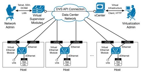
Figure 6-6 Cisco Nexus 1000V Architecture
