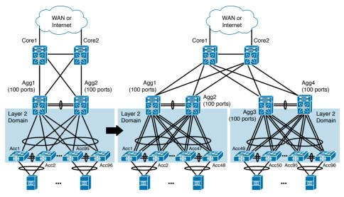
Figure 10-35 Scaling a Core-Aggregation-Access Network
