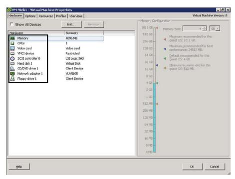
Figure 5-6 Virtual Hardware in a VMware ESXi VM
