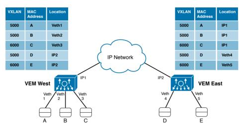
Figure 6-18 Cisco Nexus 1000V VXLAN Topology
