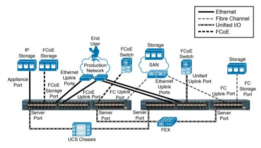
Figure 12-8 Back Panel UCS Fabric Interconnect Connections
