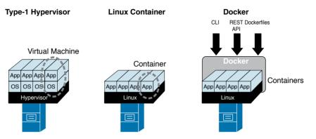
Figure 5-20 Comparing Virtual Machines, Linux Containers, and Docker
