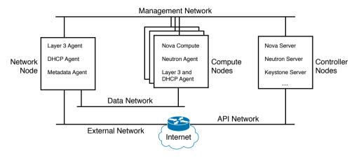
Figure 11-22 Typical Neutron Deployment
