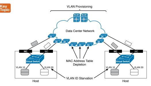
Figure 6-11 VLAN Challenges for Server Virtualization
