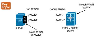
Figure 8-17 Fibre Channel World Wide Names
