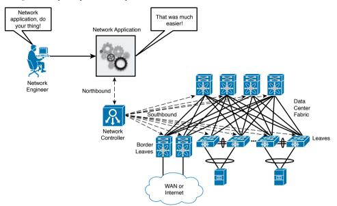
Figure 11-5 portrays the concept of a network controller in more detail.
