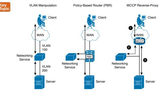
Figure 7-1 Traffic Steering Techniques in Physical Networks
