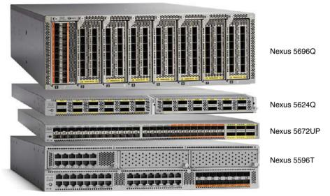
Figure 13-4 Cisco Nexus 5000 Series Switches
