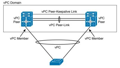
Figure 10-8 Virtual PortChannel Elements
