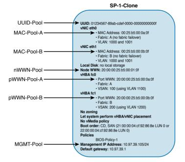
Figure 12-25 Deploying Pools with SP-1-Clone
