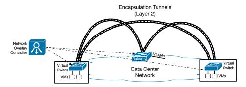
Figure 11-11 Software-based Virtual Overlay Architecture
