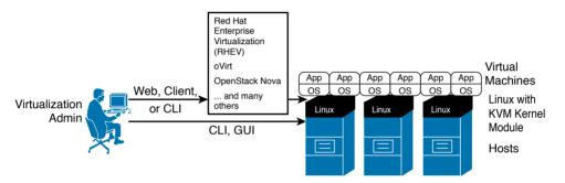
Figure 5-11 Linux KVM Architecture
