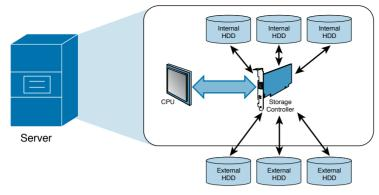
Figure 8-5 Storage Controller in a Server
