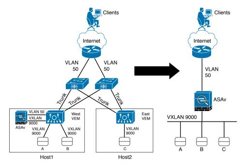
Figure 7-7 ASAv Deployment Example
