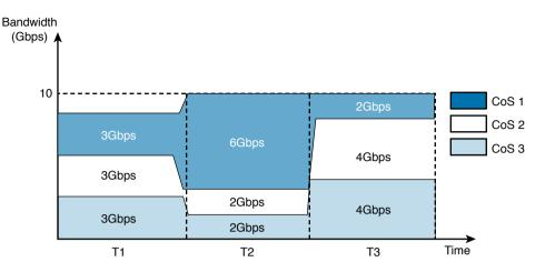
Figure 10-23 Enhanced Transmission Selection in Action
