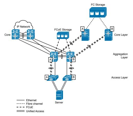
Figure 10-29 Converged Aggregation and Access Model
