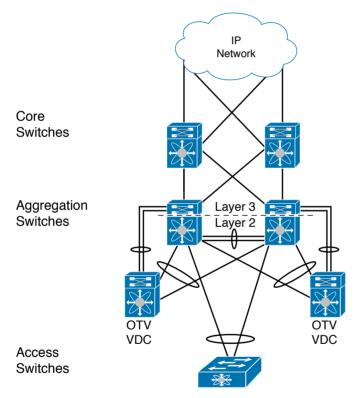
Figure 10-20 OTV Design in a Single Aggregation Switch Pair
