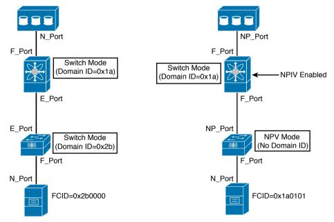
Figure 8-24 Comparing ISLs to NPV Connections
