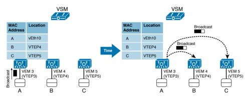
Figure 6-21 Enhanced VXLAN Head-End Replication
