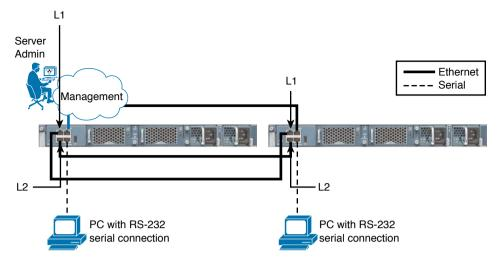
Figure 12-7 Front Panel UCS Fabric Interconnect Connections
