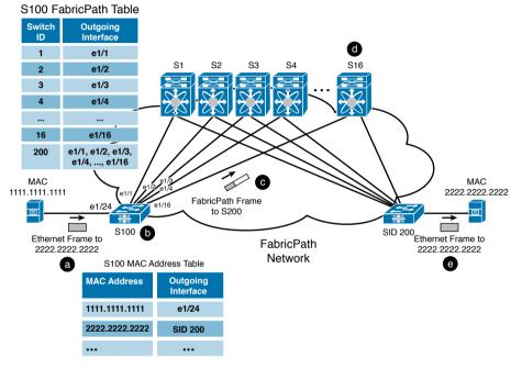
Figure 10-30 *Ethernet Frame Forwarding over a FabricPath Network*
