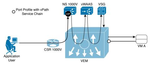
Figure 7-13 vPath Service Chain in Action
