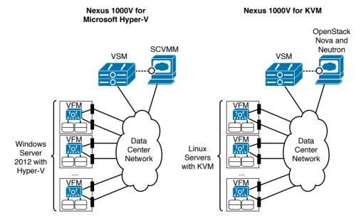
Figure 6-10 delineates the architecture of Nexus 1000V for Microsoft Hyper-V and Nexus 1000V for Linux KVM.
