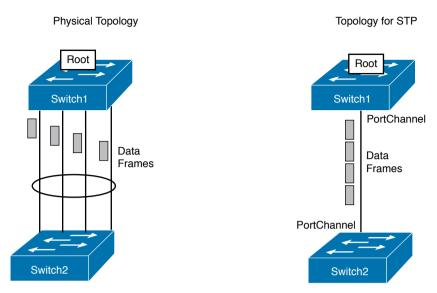
Figure 10-6 Link Aggregation Between Two Ethernet Switches
