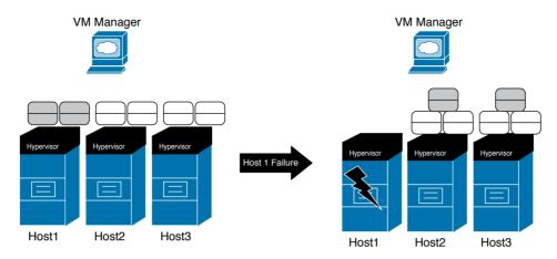
Figure 5-12 Virtual Machine High Availability Example
