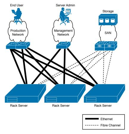
Figure 12-4Provisioning Rack-mountable Servers
