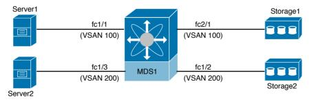
Figure 8-25 Two VSANs in a Single Switch
