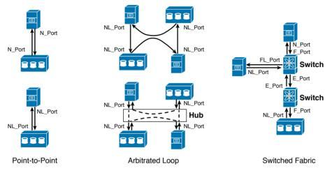
Figure 8-16 Fibre Channel Topologies
