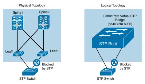
Figure 10-33 FabricPath Network from an STP Device Perspective
