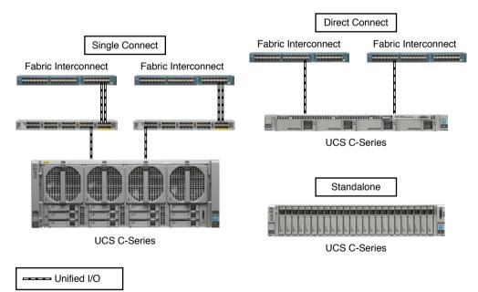
Figure 12-15 demonstrates how a UCS C-Series server can be deployed and managed.
