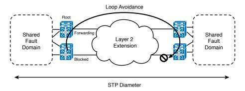
Figure 10-16 STP Challenges in Data Center Interconnections
