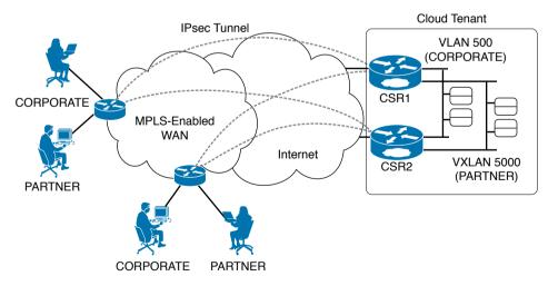
Figure 7-8 CSR 1000V Deployment Example
