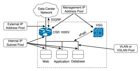
Figure 7-16 Three-tier Container Template in VACS
