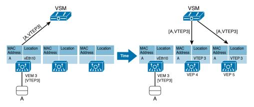
Figure 6-20 details the Enhanced VXLAN MAC address learning in Nexus 1000V.
