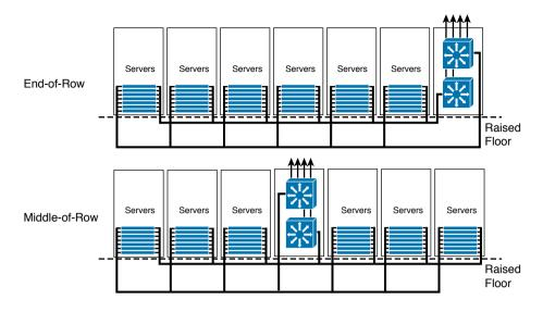
Figure 10-11 End-of-Row and Middle-of-Row Topologies
