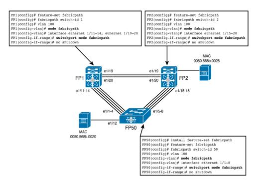
Figure 10-32 FabricPath Configuration Example
