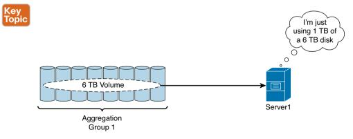
Figure 8-9 Thick Provisioning
