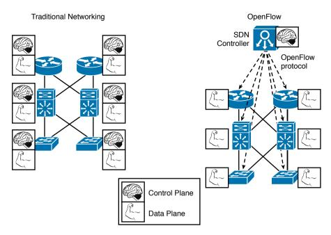
Figure 11-6 Separating Control and Data Planes
