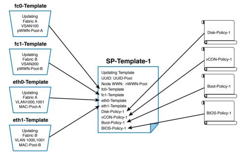
Figure 12-26 Service Profile Template Example
